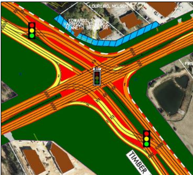
CFI intersection design from TIP project U-5744 public meeting – image from NCDOT website
