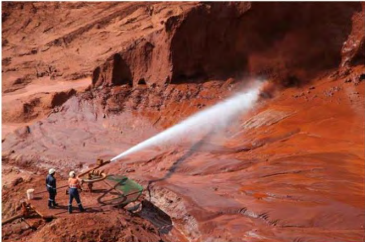
Figure 4.1 Base Kwale Hydraulic Mining
