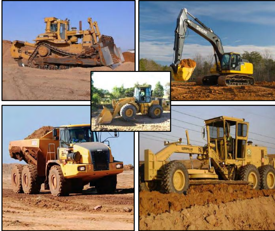
Figure 25: Dozer, excavator, tipper, grader and front end loader earth moving equipment.
