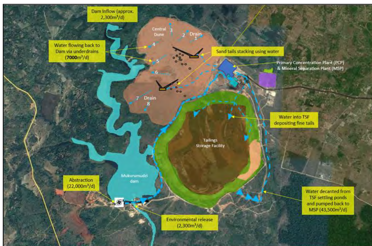
Figure 2-1: General Layout of Base Mine Site and Water Flows
