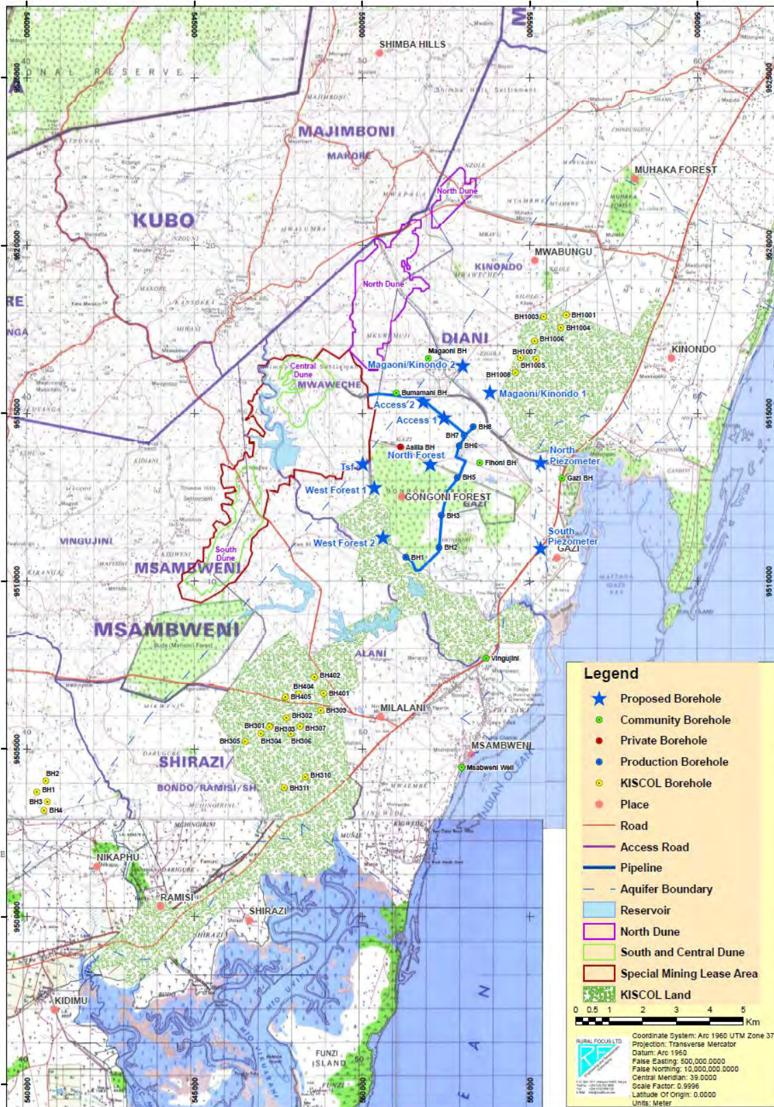
Figure 3.3 : General locations of additional boreholes and piezometers
