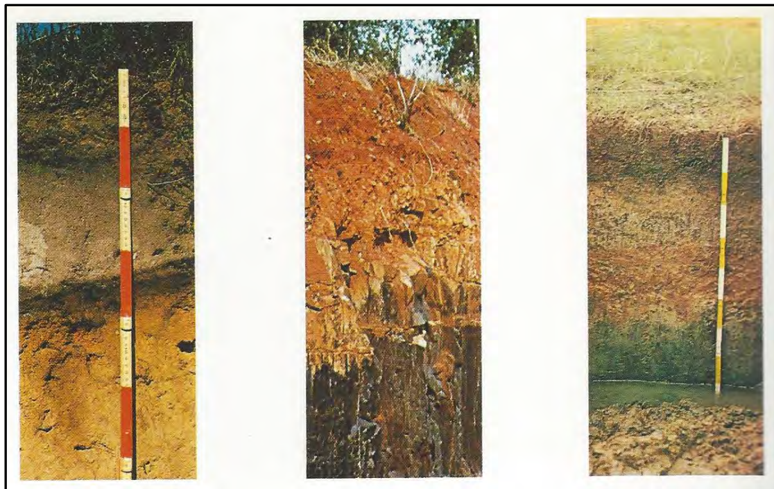
Figure 4. Soil systems with different layers, Left: Orthic A-Horizon/Podzol B-Horizon/Rock, Middle: Orthic A-Horizon/Rock, Right: Orthic A-Horizon/E-Horizon/Soft Plinthic B-Horizon (Schroeder, 1984).
