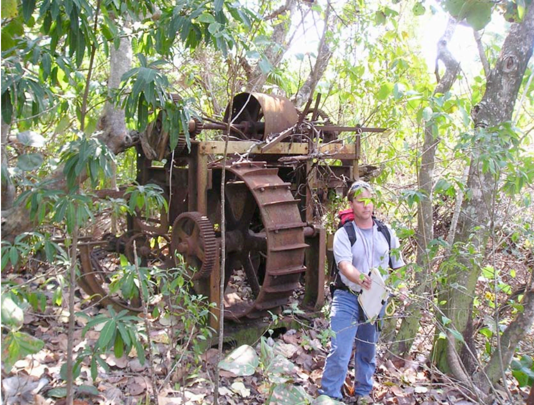
Photo of sisal plantation ruins on Great Guana Cay: This machinery may be one of the few early mechanical mills used to clean the fiber from sisal plants for export. The location of this photo is:
