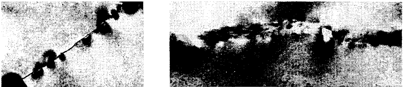
Figure 9 TEM images of SiO 2 and SiC precipitates at grain boundaries (left) and dislocations (right) in RGS ribbon solar cells.
