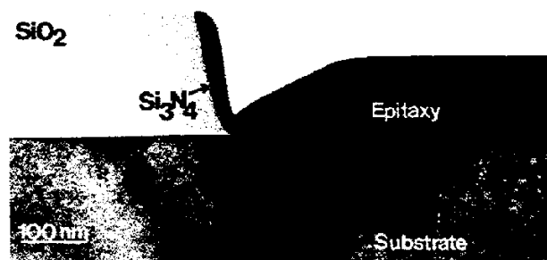
Figure 1. Epitaxial layer selectively grown by UHV-RTCVD using Si 2 H 6 /Cl 2 chemistry
