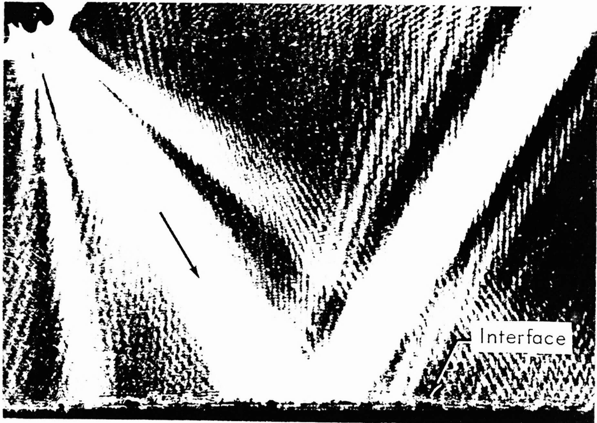
Figure 2. The effect of transducer sidelobes on a photograph of the reflection of an ultrasonic wave at an interface.
