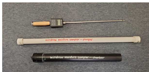
Figure 14-2. An electronic bale moisture probe cannot measure the moisture content of loose hay. Using a windrow moisture sampler to compact the hay sample makes rapid moisture testing before baling possible.
