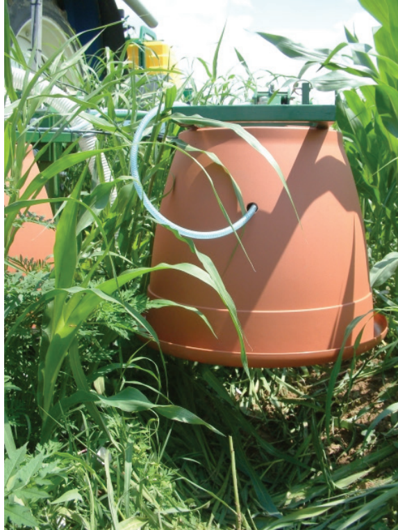
Figure 1. WeedSeeker sensor-sprayers shielded by plastic container
