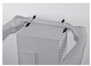
Figure 8-3: Separate Cover And Back
