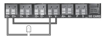
Figure 8-16: Output Relay with Internal 24 Volt Supply
