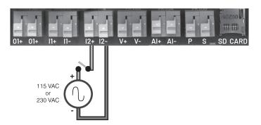
Figure 8-15: External Input with External Supply
