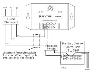
Figure 11-1: SPP233 Standard Control Box Connection
