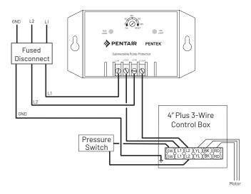
Figure 11-2: "Plus" Control Box Connection for SPP233
