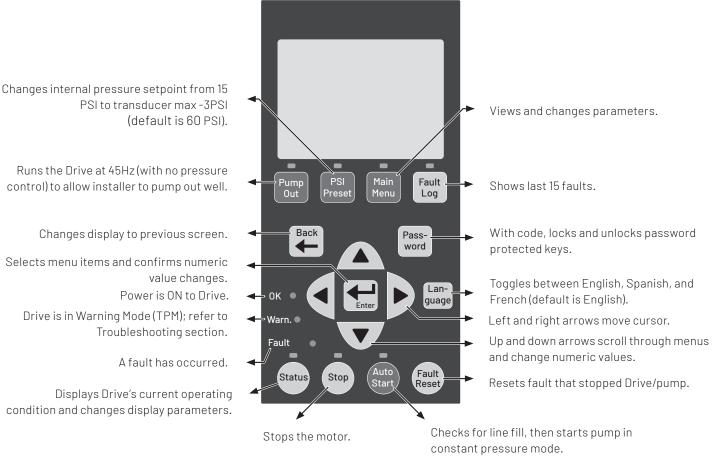
Figure 8-2: Pentek Intellidrive Keypad Functions
