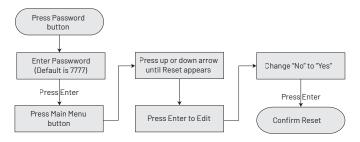
Figure 8-18: Keypress Sequence For Testing
