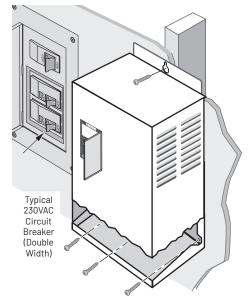
Figure 8-6: Separate Cover And Back
