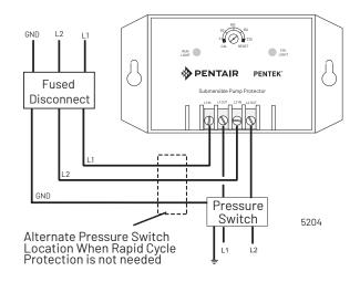
Figure 11-3: Two-Wire Connection for SPP233
