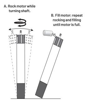
Figure 6-2: Rock Motor gently from side to side while turning shaft by hand (A), then fill with clean water (B). Repeat until full.
