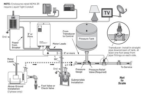
Figure 8-1: A typical residential installation layout
