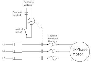
Figure 4-9: Separate Voltage Control
