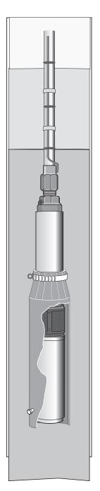
Figure 5-2: Flow Inducer Sleeve
