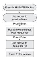
Figure 8-10: Select 80 Hz (Three-phase submersible operation only)
