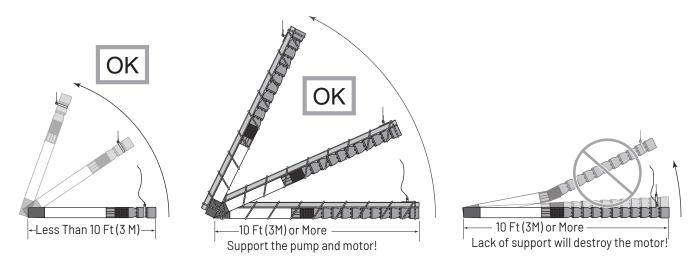
Figure 6-1: When the pump and motor together (without any riser pipe) are 10ft (3m) long or more, support the assembly before lifting to avoid bending it in the middle. Never try to lift the motor or pump by the motor cables.
