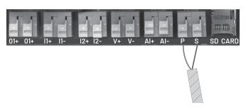
Figure 8-17: Example RS-485 Connection
