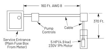
Figure 4-1: Mixing Wire Sizes Example
