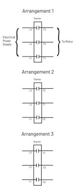
Figure 4-11: Example of Three-Phase Current Unbalance
