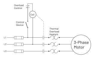
Figure 4-7: Line Voltage Control
