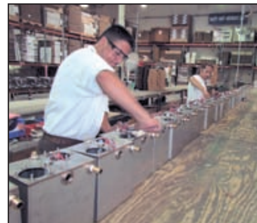
Employees assemble steam-shower generators from components that are designed specifically for ThermaSol products.
