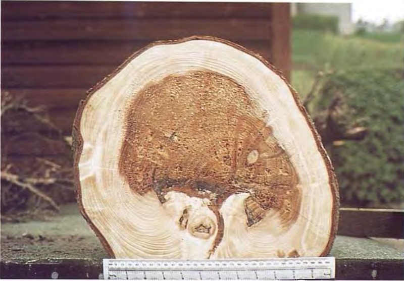
Fig 68. Wound rot in Sitka spruce. The original wound surface, parts of which can be seen in the lower half of the section, has been obscured by healing growth pushing into the rotted area.
