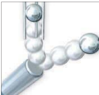
Mechanical protection of electronic part proven in ball drop test
