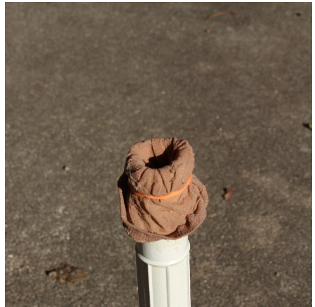
Figure 2. Collect and remove ladybugs and other invaders without contaminating your vacuum cleaner by intercepting the insects with an inverted sock attached to the tube with a rubber band.
