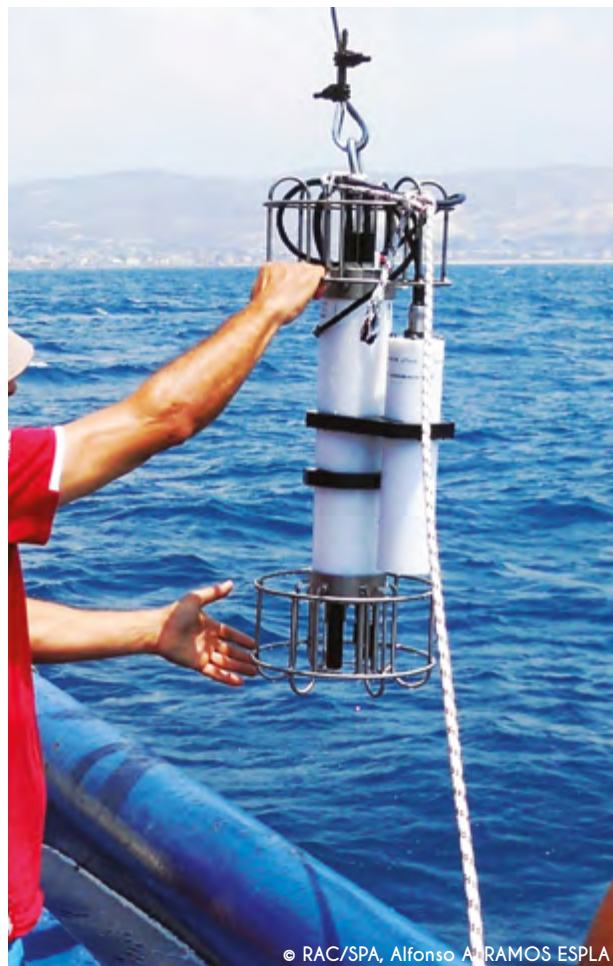
Figure 10. Launching the TCD off the stern of the oceanographic boat 'CANA'
