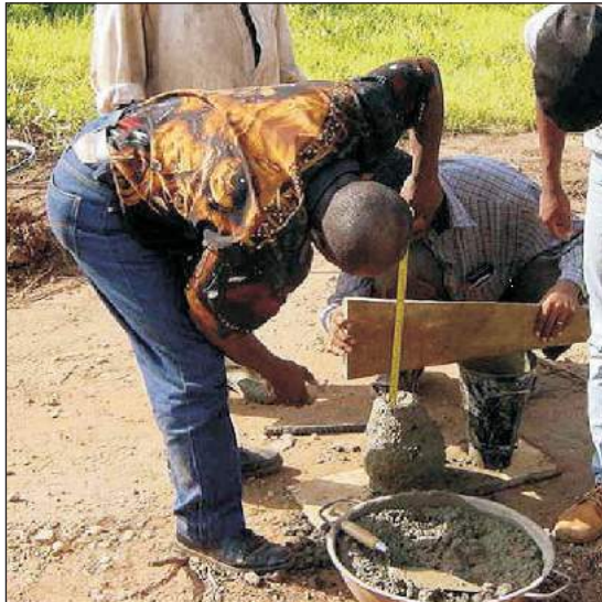
Figure C.8.10: Workable and cohesive concrete
