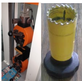
Figure 2. Electromechanical universal test machine for adhesion test and cut tool for glue
