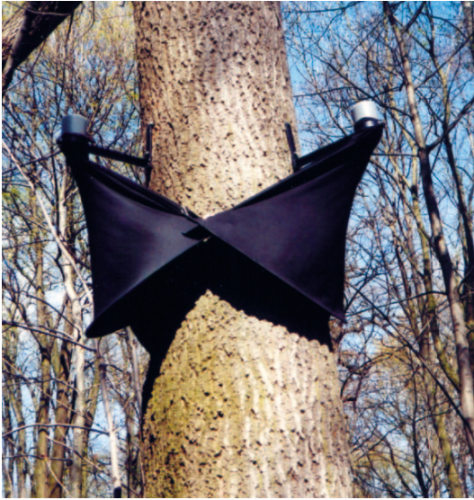
Figure 3 – Stem elector fixed around a large Tilia cordata tree in about 3 m in height.
