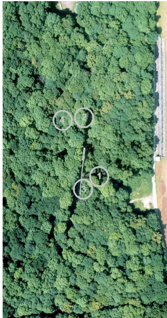
Figure 4 – Aerial view of the crane range, crane rail track (length: 120 metres), location of control units 1 to 4: unit 1: Forest SE – a canopy depression; unit 2: Rail track N – an approximately 5 m broad vertical channel; unit 3: Rail track S – the crane rail track is in a 10 to 15 m wide forest gap; unit 4: Forest NW – a recent clearing in the forest, due to a huge oak tree blown down in a heavy storm.
