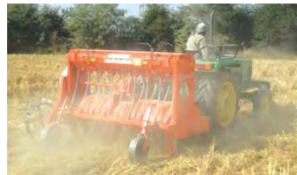
Fig. 16. A 'Happy Seeder' for direct drilling of seeds in presence of surface residues (Courtesy: CSISA, CIMMYT-IRRI, New Delhi)
