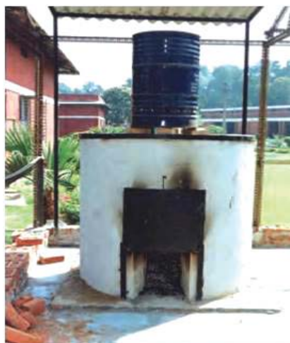
Fig. 14. Low-cost pyrolysis kiln for preparation of biochar (Courtesy: T.J. Purakayastha, IARI, New Delhi)
