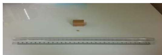
Figure 2. The micro- and standard-size tension (upper) and compression (bottom) test samples
