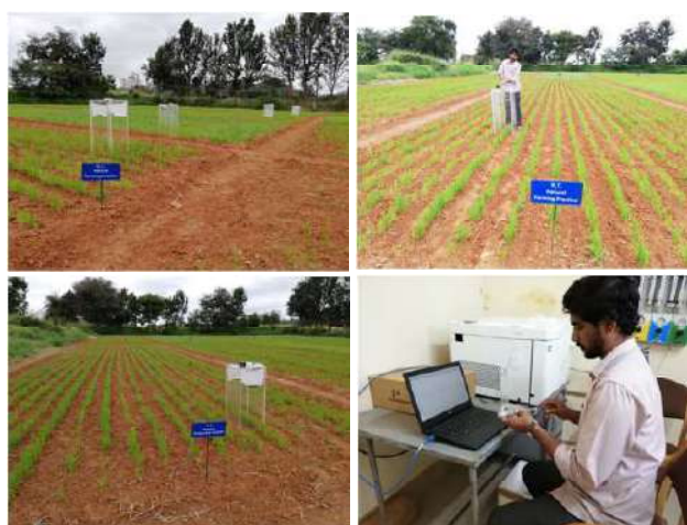
Plate 1: Collection of methane and nitrous oxide gases placed in the research plots using closed chamber technique and estimation of gases by using GCMS instrument
