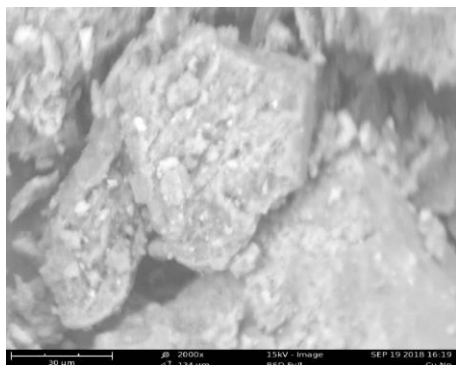
Figure 6: Zoomed SEM image of copper nanoparticles
