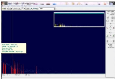
Figure 10: Showing Maestro-32 spectrum analysis (peak info and pulse height analysis) of pacemaker P10 after exposure to radiation
