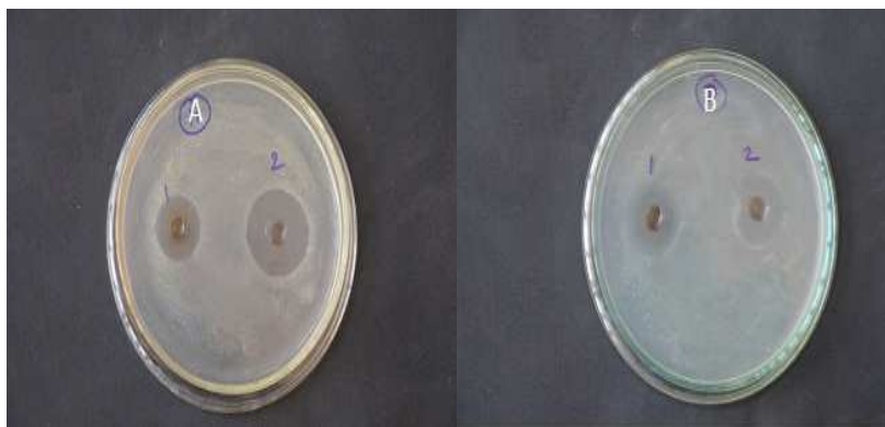
Fig-4 Antibacterial activity of silver nanoparticle against (A) Bacillus subtilis (B) Staphylococcus sp. In each image (1)AgNPs (2)Streptomycin antibiotic
