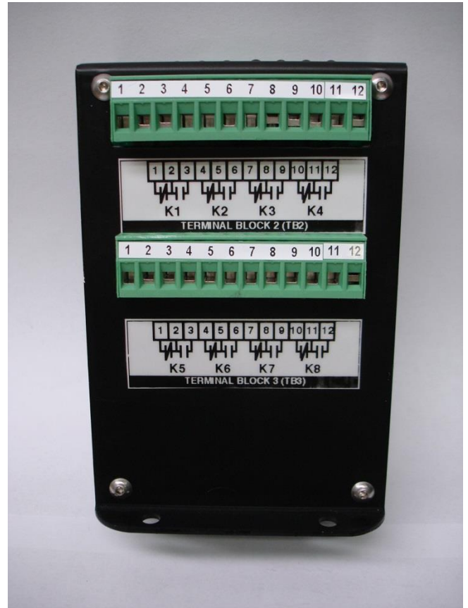
TB 2 AND TB 3 (RELAY CONTACT WIRING)
