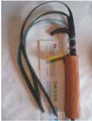
Fig. 1 - A mimic of a Posidonia oceanica shoot used in this study.
