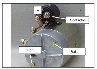
Figure 3-3: DC motor showing contactor and bolt location.
