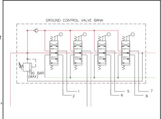
Figure 3-10: Ground control valve.
