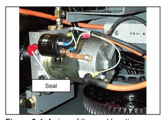
Figure 3-4: A view of the seal location.
