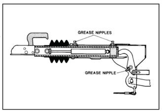
**Figure 3-33**: View of the grease nipple locations.
