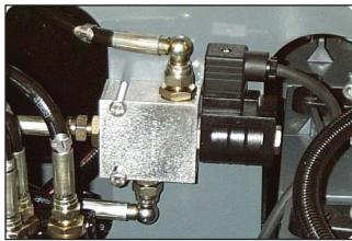
Figure 3-25: Diverter valve.
