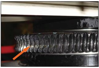
**Figure 3-37**: Location of the slew drive gears.
