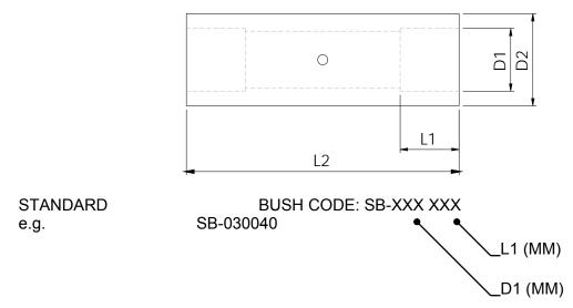
THE BUSH MUST FILL THE COMPLETE LENGTH OF L1. HOWEVER, IT IS ACCEPTABLE TO MAKE UP THR TOTAL LENGTH L1 BY USING MORE THAN ONE BUSH
