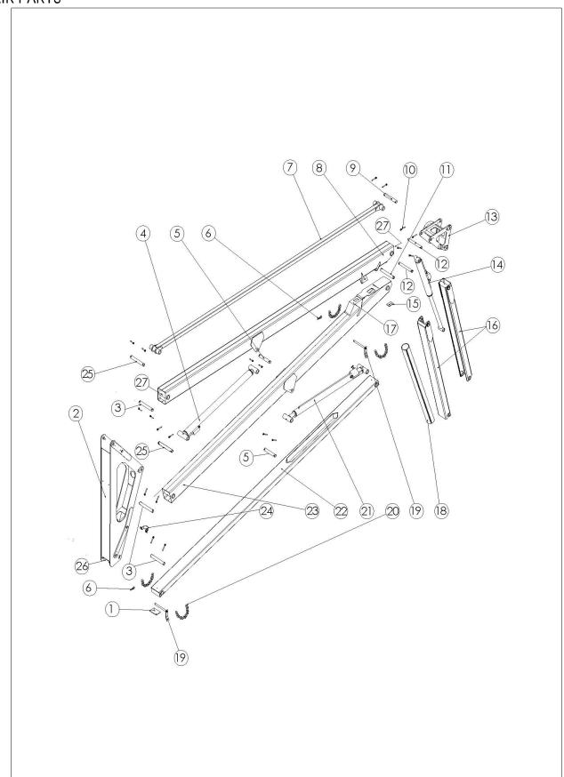
TL37J PARTS MANUAL BOOM ASSEMBLY PARTS
