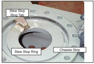
Figure 3-39: Critical parts of the slew stop.
