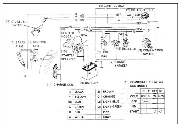
Figure 3-18: Engine engine schematics.
