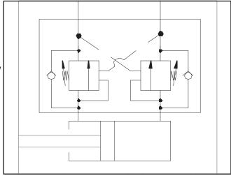
Figure 3-7: Dropnose cylinder with welded on block containing 2 adjustable O/C valves.
