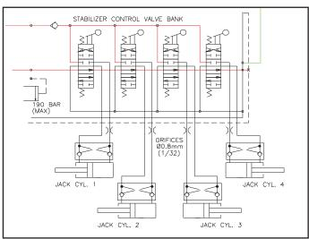
**Figure 3-12**: Schematic view of outrigger control valve.
