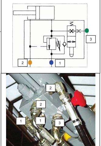
Figure 3-6: For clarity, the drawing shows only one hose to each service. In reality, there are two hoses. One for the platform controls and one for the ground controls. Only the emergency lower has one hose.
