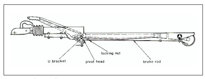
En-Figure 3-32: Coupling/Overrun device. sure that the draw bar is fully extended. Screw the brake rod into the pivot head and secure with an M10 nut. Using the M10 ball nut, connect the brake rod to the Bowden cable via the compensating bracket. Fit and hand tighten the hex securing nut. Tighten the M10 ball nut on the brake rod until there is no further play on the pivot head against the draw bar (the draw bar must be fully extended).
