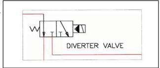
Figure 3-11: Diverter valve schematic.
