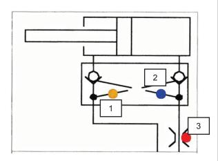
**Figure 3-8**: Outrigger cylinder with welded on block containing the two check valves. The restrictor shown is the hose adaptor fitted in the outrigger control valve.
