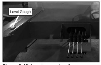
Figure 3-19: Level gauge location.
