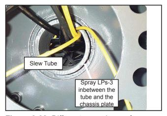
**Figure 3-38**: Different procedures of lubrication.
