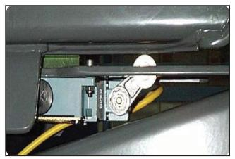
Figure 3-24: Boom limit switch.
