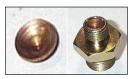
**Figure 3-14**: Copper restrictor fitted loose in the hose adaptor. Hose end requires more torque to prevent oil leak when securing hose.
