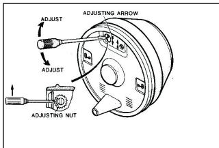
Figure 3-30: Nut adjusting direction.
