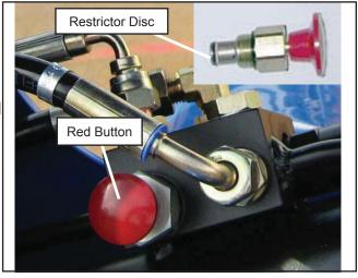
**Figure 3-5**: A view of the manual release valve and restrictor disc.
