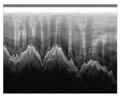
**Fig. 2.3** A radar image of the Gamburtsev Mountains showing the jagged mountain range covered in layers of ice (With kind permission from the AGAP project, Lamont-Doherty Earth Observatory of Columbia University)
