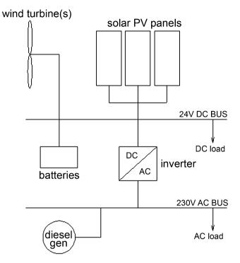
Fig. 26.3 This line diagram shows a renewable electricity system (© Pat Bodger)
