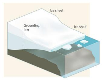
Fig. 5.10 The main features of an Antarctic ice shelf (Reprinted with kind permission from Macmillan Publishers Ltd: Nature, from Huybrechts 2009)
