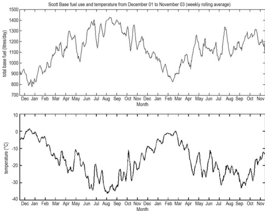
**Fig. 26.7** The *top panel* shows the total amount of fuel used at used at New Zealand’s Scott Base, from December 2001 to November 2002. The *lower panel* shows the temperature in °Celsius (°C) (Pat Bodger)
