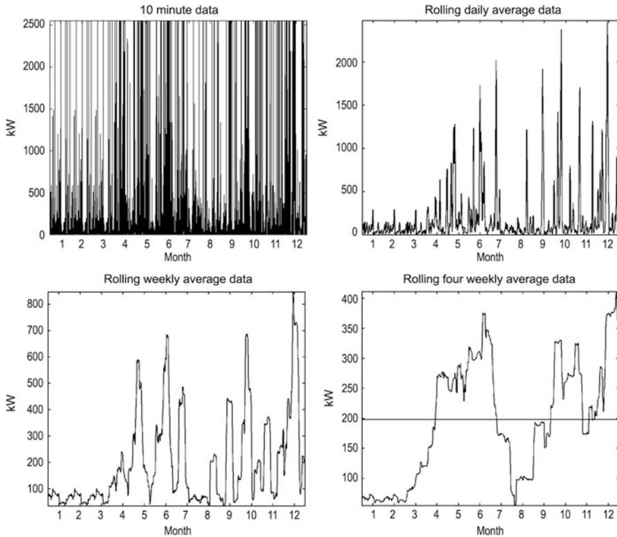
**Fig. 26.12** Power output of a Ropatec 3 kVA vertical axis wind turbine (© Pat Bodger)
