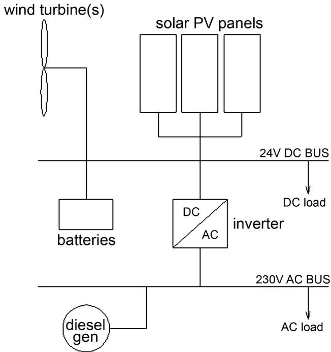
Fig. 26.3 This line diagram shows a renewable electricity system (© Pat Bodger)
