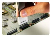
E5385A 34-channel Samtec connector probe
