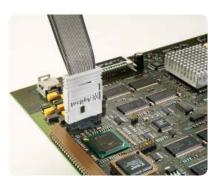
E5346A 34-channel Mictor connector probe
