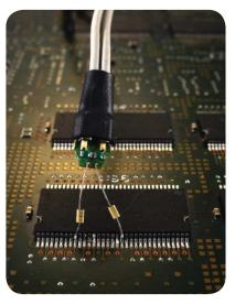
InfiniiMax solder-in probe head with long wires
