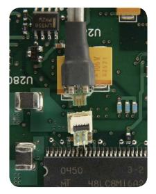
InfiniiMax ZIF tip soldered on board
