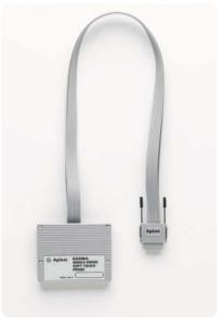
E5396A 16-channel soft touch connectorless probe
