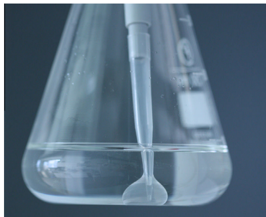
Fig. 1. Separation of benzyl benzoate from the culture medium using a micropipette.
