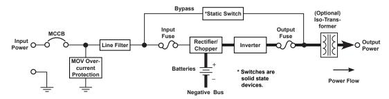
FIGURE 12.5: POWER FLOW IN BATTERY BACKUP FOR ALL MODELS
