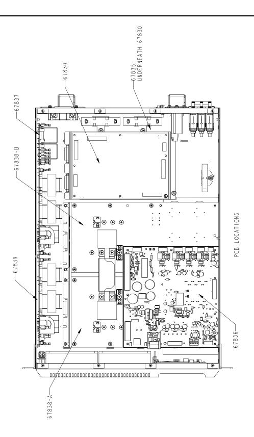
FIGURE C-4: T1000 POWER MODULE - PCB LOCATIONS
