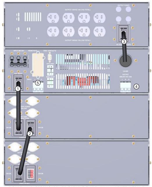
FIGURE 7.6: FACTORY SUPPLIED CABLING GUIDE - W/ 120V XFMER MODULE TABLE 7.5: 120V SYSTEM CABLING SPECIFICATIONS
