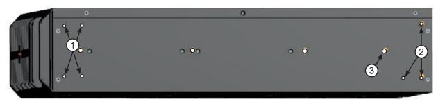
FIGURE 6.8: RACKMOUNT BRACKET MOUNTING HOLES
