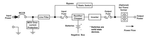
FIGURE 12.4: POWER FLOW AFTER AN EPO COMMAND FOR ALL MODELS
