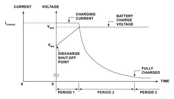
FIGURE 12.7: BATTERY RECHARGING PROFILE
