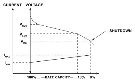
FIGURE 12.6: BATTERY DISCHARGE CURVES
