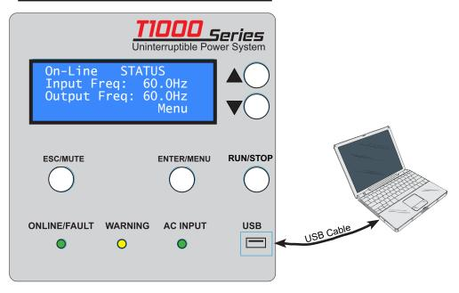
FIGURE 15.4: CABLING THE T1000 TO A PLATFORM RUNNING THE "TOSHIBA T1000 SERIES UPS MONITORING PROGRAM"
