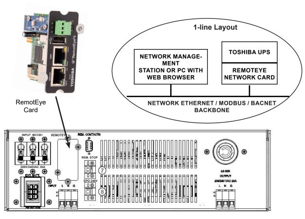
FIGURE 15.2: REMOTEYE INSTALLATION
