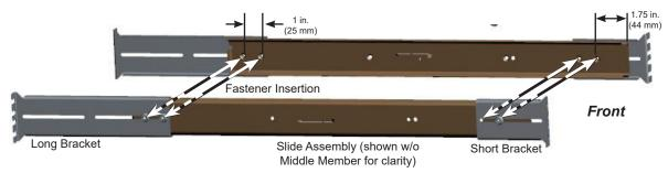
FIGURE 4: ATTACH EXTENDER BRACKETS TO SLIDE ASSEMBLY
