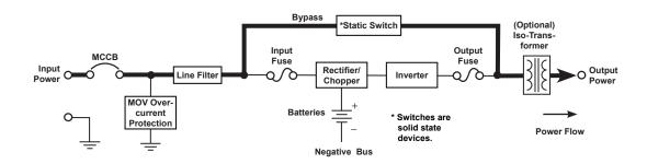
FIGURE 12.1: POWER FLOW IN BYPASS FOR ALL MODELS
