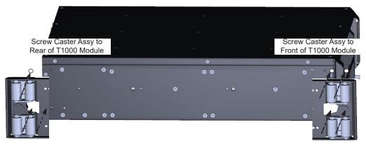
FIGURE 4: ATTACH CASTER ASSEMBLIES
