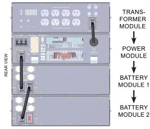
FIGURE 6.2: RACKMOUNT 120V<sub>OUT</sub> SYSTEM WITH TRANSFORMER MODULE
