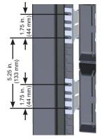
FIGURE 5 CAGE NUT INSTALLATION
