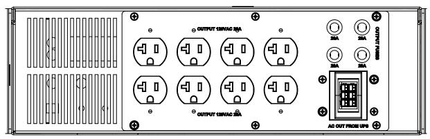
FIGURE 7.5: TRANSFORMER MODULE - BACK PANEL LAYOUT
