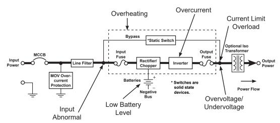
FIGURE 16-1: UPS PROTECTION DEVICE LOCATIONS
