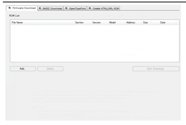
Be sure to avoid the environment where a power failure may occur in the middle of the downloading. If a power failure occurs during a firmware updating, the printer may not start up. Even when the printer can normally start up, download the firmware again.
