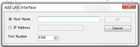
After the value is filled in and [OK] is clicked, the dialog box is closed and the setting is reflected in the interface list.
