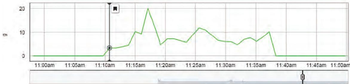
Graph indicates high and variable overall acceleration, an indication of potential cavitation.
