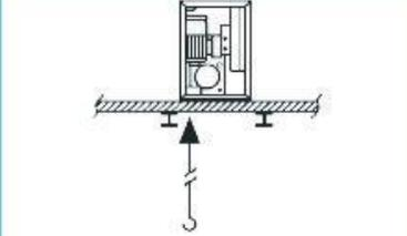
If the opening is not large enough for the hook, first position the hoist and guide the wire rope with the tip through the opening and into the Tirak™.
