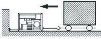
Secure the mobile hoist to a suitable anchor point by using a sling, chain or other securing method and you will be ready to start working.
