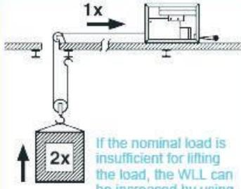
If the nominal load is insufficient for lifting the load, the WLL can be increased by using a number of blocks/ sheaves.
