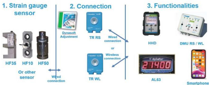
1. Select or design a strain gauge sensor that fits perfectly in your application. Tractel offers standards sensors as well as specific sensors.
