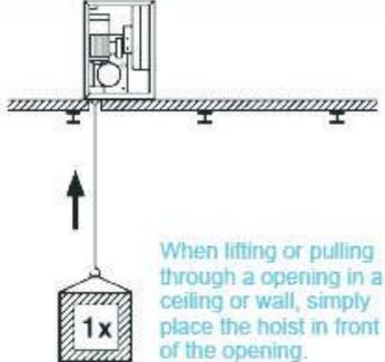
When lifting or pulling through a opening in a ceiling or wall, simply place the hoist in front of the opening.
