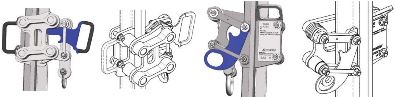
The Safety parking clamps (SPC) are dedicated to securing lifting platforms used in the elevator industry by attaching the platform to the guiding rail. They are used as a secondary safety device, a primary safety device is mandatory.
