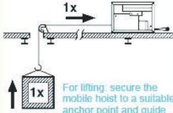
For lifting: secure the mobile hoist to a suitable anchor point and guide the wire rope through 1 or more sheave blocks.
