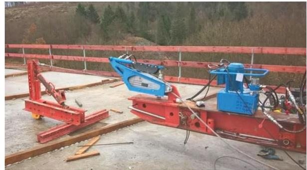
The Tirfor TU-A16 and TU-A32 can be motorized by a pneumatic system powered by an onsite or portable air supply and is operated by a standard control unit.
