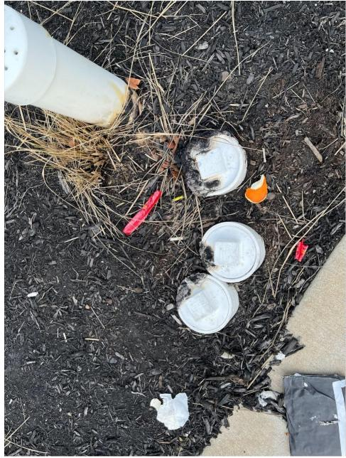
Apparent evidence of fire in mulch. PVC pipes charred and melted.
