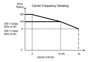
Figure A.1 Carrier Frequency Derating
