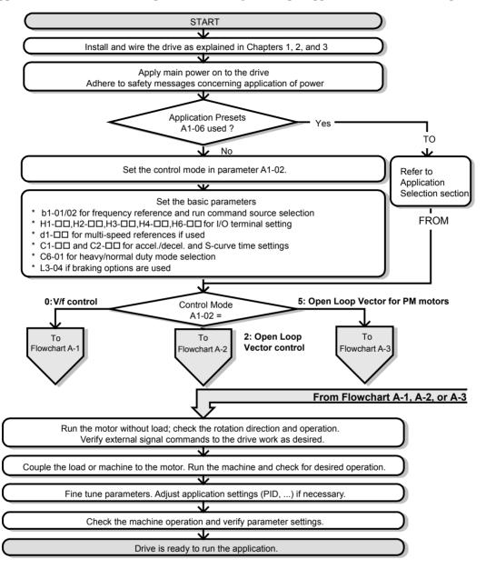
Figure 4.6 Basic Start-up and Motor Tuning
