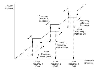
Figure 5.33 Jump Frequency Operation
