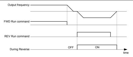
Figure 5.63 Reverse Direction Output Example Time Chart
