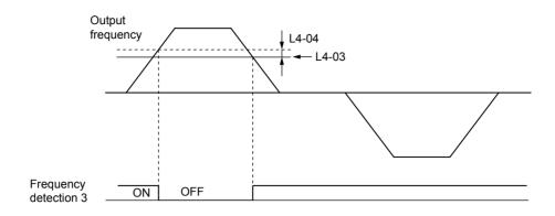
Figure 5.61 Frequency Detection 3 Example with Positive L3-04 Value
