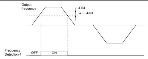
Figure 5.62 Frequency Detection 4 Example with Positive L3-04 Value
