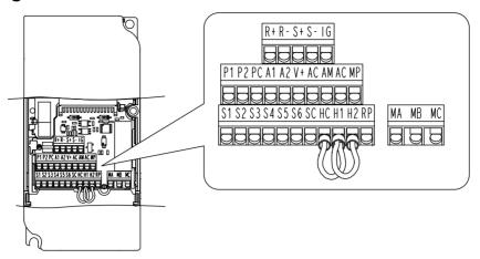
Figure 3.16 Removable Control Circuit Terminal Block
