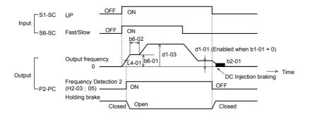
Figure 4.12 Holding Brake Time Chart
