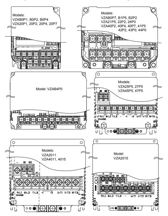
Figure 3.5 Main Circuit Terminal Block Configurations
