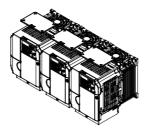
Figure 2.4 IP20/NEMA 1 Side-by-Side Mounting in Enclosure
