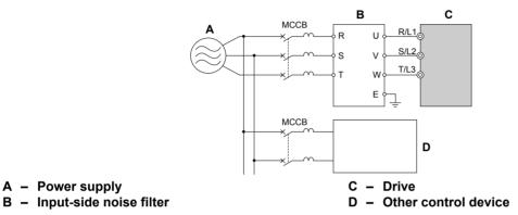
Figure 8.6 Input-Side Noise Filter (Three-Phase 200/400 V)
