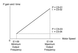
Figure 5.28 Adjusting ASR Proportional Gain and Integral Time
