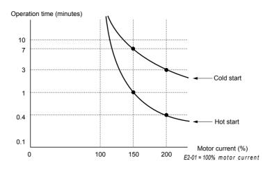
Figure 5.74 Motor Protection Operation Time
