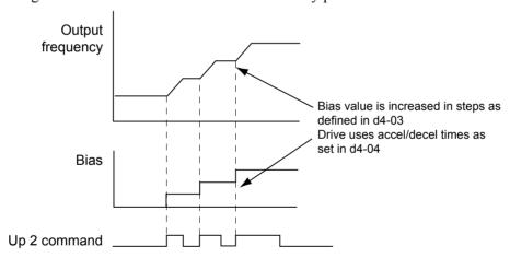
Figure 5.38 Up/Down 2 Bias when d4-03 > 0.0 Hz
