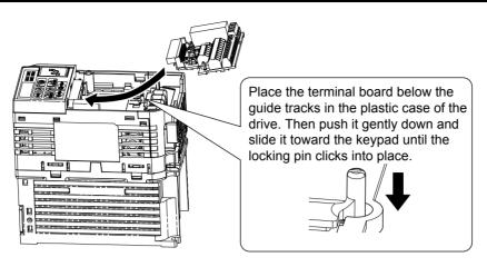
Figure 7.9 Terminal Board Replacement
