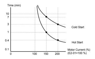
Figure D.8 Motor Overload Protection Time
