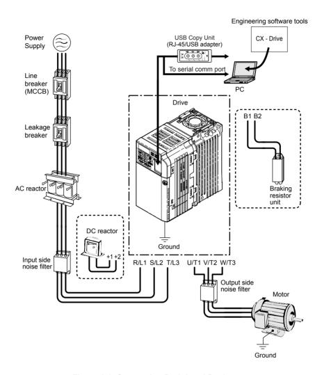
Figure 8.1 Connecting Peripheral Devices
