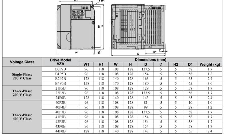
Table 2.5 IP20/Open-Chassis (with EMC filter)
