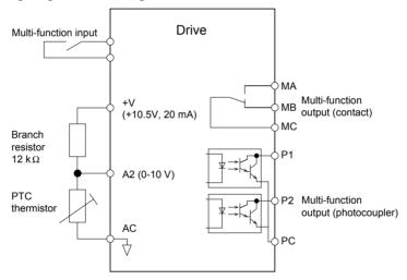
Figure 5.75 Connection of a Motor PTC
