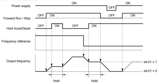
Figure 5.34 Frequency Reference Hold with Accel/Decel Hold Function
