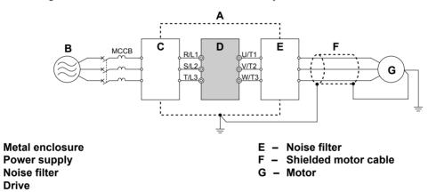
Figure 8.9 Reducing Radio Frequency Noise
