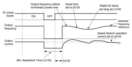
Figure 5.14 Current Detection Speed Search after Power Loss
