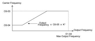
Figure 5.29 Carrier Frequency Changes Relative to Output Frequency
