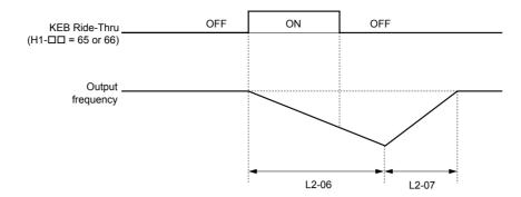
Figure 5.77 KEB Ride-Thru Timing Diagram for Multiple Drives
