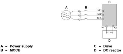
Figure 8.4 Connecting a DC Reactor
