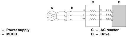
Figure 8.3 Connecting an AC Reactor
