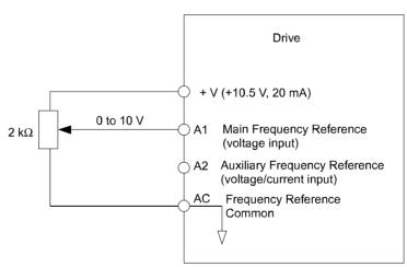
Figure 5.1 Setting the Frequency Reference by Voltage Input
