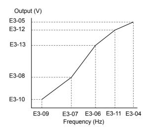
Figure 5.41 V/f Pattern for Motor 2
