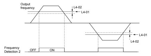
Figure 5.58 Frequency Detection 2 Time Chart
