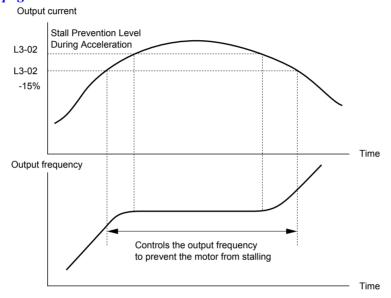
Figure 5.79 Stall Prevention During Acceleration for Induction Motors
