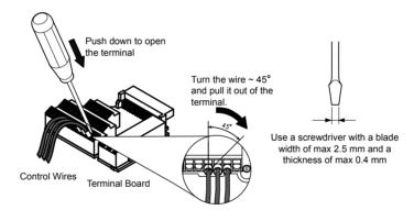
Figure 3.19 Removing Wires from the Terminal Board
