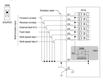
Figure 3.23 Sinking Mode: Sequence from NPN Transistor (0 V Common)
