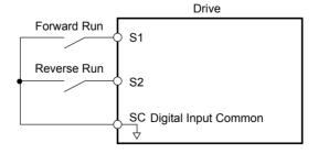
Figure 5.51 Example Wiring Diagram for 2-Wire Sequence
