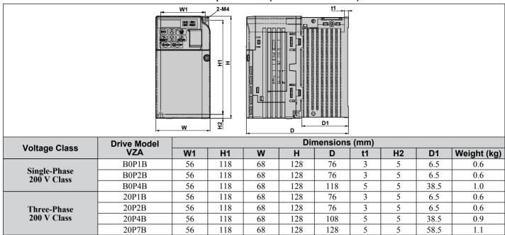
Table 2.4 IP20/Open-Chassis (without an EMC filter)
