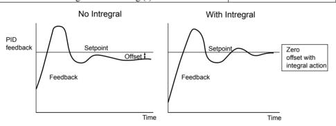
Figure 5.19 Offset Elimination by Integral Operation
