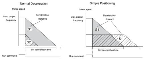
Figure 5.10 Simple Positioning Deceleration
