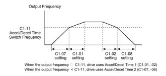
Figure 5.24 Accel/Decel Time Switching Frequency
