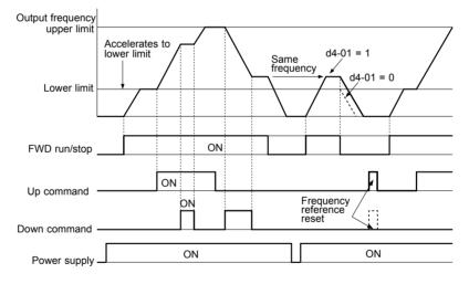
Figure 5.46 Up/Down Command Operation
