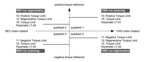
Figure 5.71 Analog Input Torque Limits
