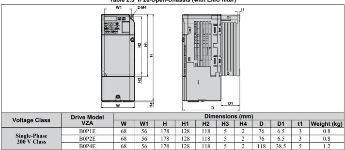
Table 2.6 IP20/Open-Chassis (with EMC filter)
