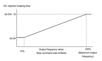
Figure 5.7 DC Injection Braking Time Depending on Output Frequency
