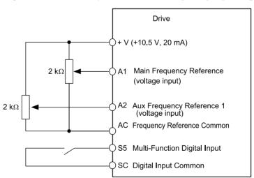
Figure 5.3 Switching between Analog Reference 1 and 2
