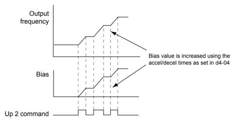
Figure 5.37 Up/Down 2 Bias when d4-03 = 0.0 Hz
