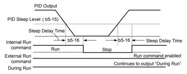
Figure 5.21 PID Sleep Operation
