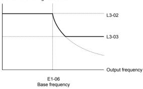
Figure 5.81 Stall Prevention Level and Limit During Acceleration
