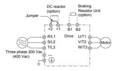
Figure 3.4 Connecting Three-Phase Main Circuit Terminals
