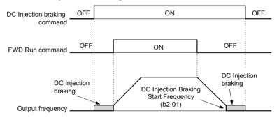
Figure 5.52 DC Injection Braking Input Timing Diagram
