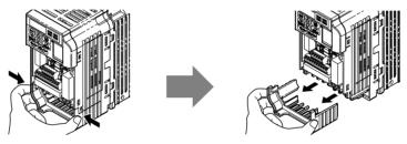
Figure 3.7 Remove the Terminal Cover on an IP20/Open-Chassis Drive
