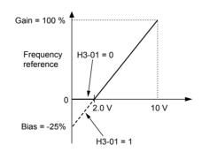
Figure 5.69 Frequency Reference Setting by Analog Input with Negative Bias
