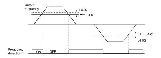
Figure 5.57 Frequency Detection 1 Time Chart
