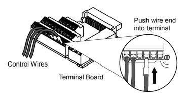
Figure 3.18 Connecting Wires to the Control Terminals
