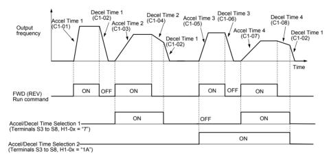
Figure 5.23 Timing Diagram of Accel/Decel Time Change
