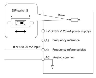
Figure 5.2 Setting the Frequency Reference by Current Input
