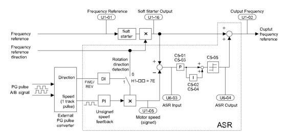
Figure 5.27 Speed Control with ASR in V/f with Simple Speed Feedback
