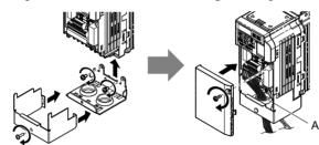
A – Pass power wiring and control signal wiring through different exit holes at the bottom of the drive. Figure 3.12 Reattach the Protective Covers and Conduit Bracket on an IP20/NEMA Type 1 Drive
