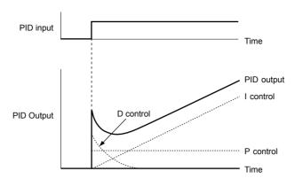
Figure 5.17 PID Operation
