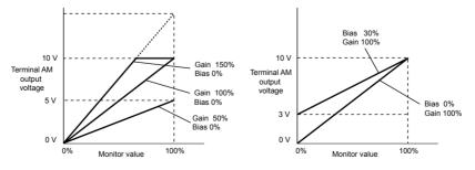
Figure 5.72 Analog Output Gain/Bias Setting
