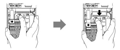
Figure 7.7 Removing the Terminal Board
