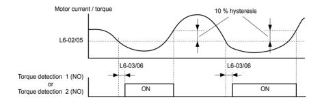
Figure 5.87 Undertorque Detection Operation
