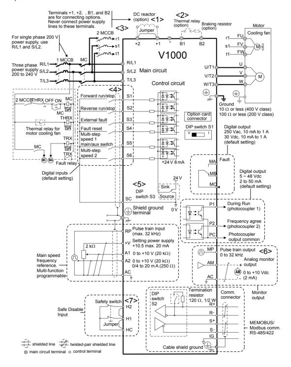
Figure 3.1 Drive Standard Connection Diagram
