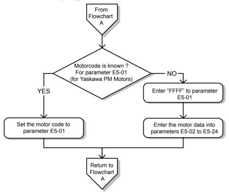
Figure 4.9 Operation with Permanent Magnet Motors
