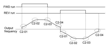
Figure 5.25 S-Curve Timing Diagram - FWD/REV Operation
