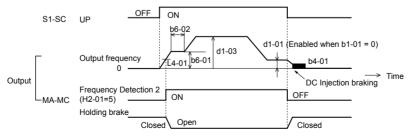
Figure 5.85 Holding Brake Time Chart
