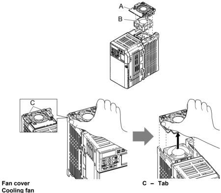
Figure 7.1 Remove the Cooling Fan Cover
