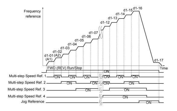
Figure 5.31 Preset Reference Timing Diagram
