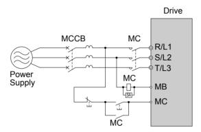
Figure 8.2 Connecting a MCCB
