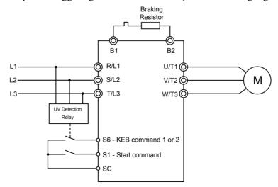
Figure 5.78 KEB Function Wiring Example
