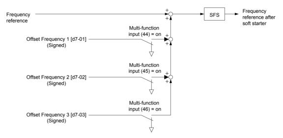
Figure 5.39 Offset Frequency Operation
