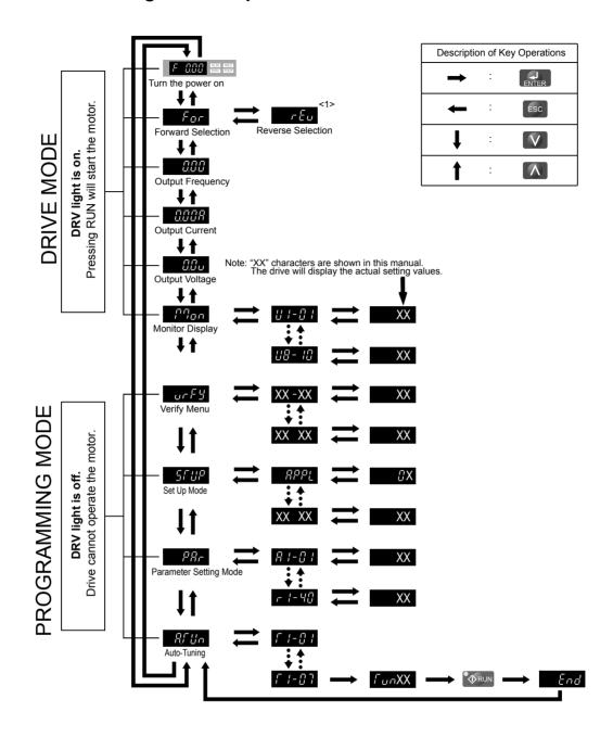
Figure 4.3 Digital LED Operator Screen Structure
