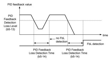
Figure 5.20 PID Feedback Loss Detection
