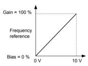
Figure 5.67 Analog Input A1 Default Characteristics
