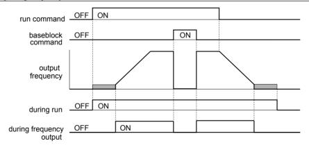
Figure 5.64 During Frequency Output Time Chart
