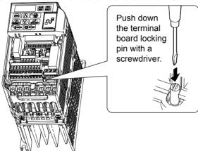
**4.** While holding down the locking pin from step 3, slide the removable terminal block in the direction of the arrows in *Figure 7.7*.
