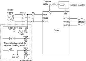
Figure 3.27 Connecting a Braking Resistor
