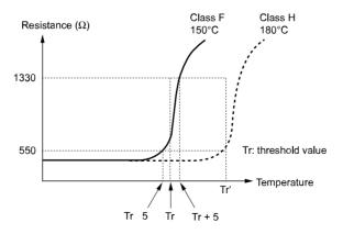
Figure 5.76 Motor PTC Characteristics
