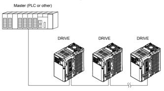
Figure C.1 Connecting Multiple Drives to a PLC
