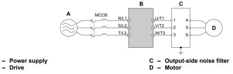
Figure 8.7 Output-Side Noise Filter
