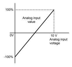
Figure 5.66 Analog Input without Limit (Bias Setting -100%)
