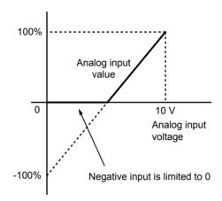
Figure 5.65 Analog Input with Limit (Bias Setting -100%)
