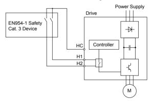
Figure D.9 Safe Disable Wiring Example
