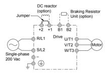
Figure 3.3 Connecting Single-Phase Main Circuit Terminals
