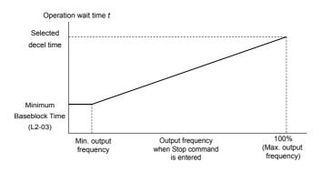
Figure 5.9 Operation Wait Time Depending on Output Frequency
