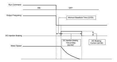
Figure 5.6 DC Injection Braking to Stop
