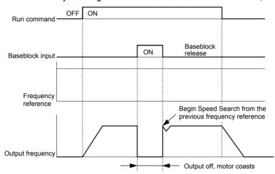
Figure 5.45 Baseblock Operation During Run
