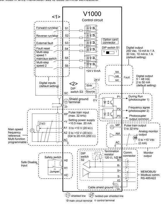
Figure 3.14 Control Circuit Connection Diagram
