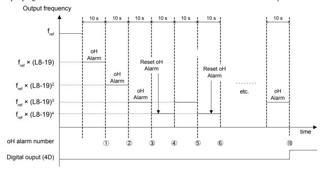
Figure 5.88 Output Frequency Reduction During Overheat Alarm
