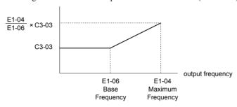
Figure 5.26 Slip Compensation Limit
