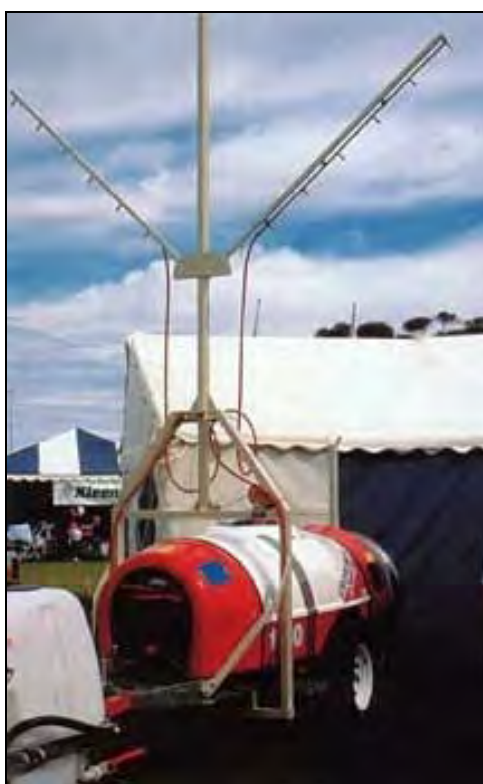
Plate 5. Structurally modified low-profile air-blast sprayers.
