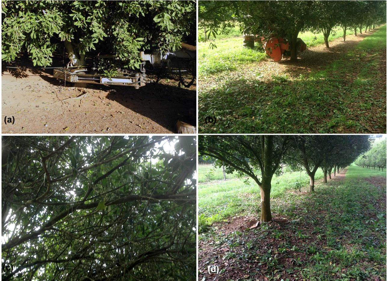
Fig. 2: Hydro-mechanical tree shakers with (a) forward and (b) backward mounted shaker clamps, (c) 100% removal of nut and stick-tights in the tree canopy and (d) damage to the trunk caused by the backward mounted clamps with nuts, stick-tights and foliage removed in the process of shaking.
