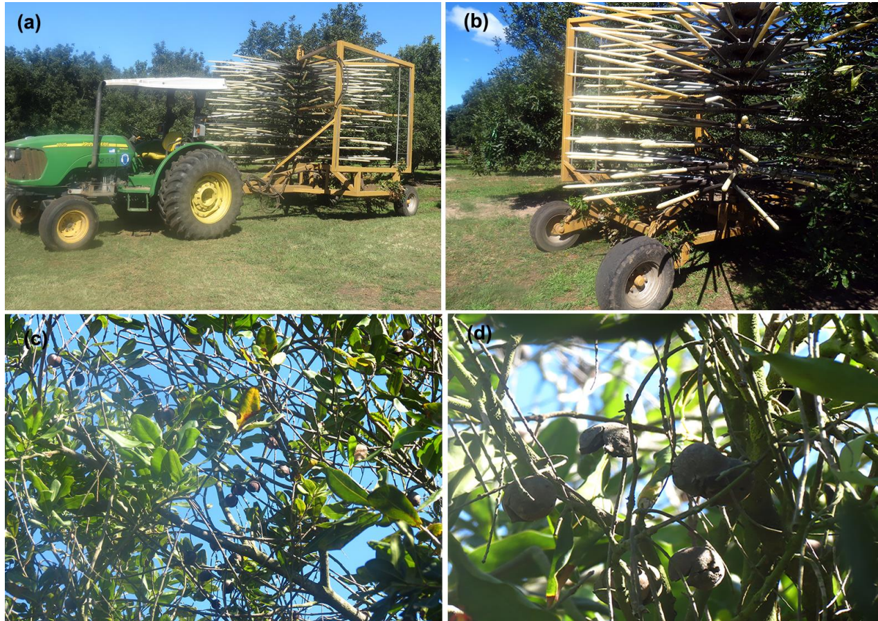
Fig. 1: (a) Tractor- mounted tree (TMT) shaker with finger-wheel-like device; (b) close up of the finger-wheel-like device in the tree canopy; (c) sticktights and (d) close up of sticktights with husk spot lesion in the tree canopy.
