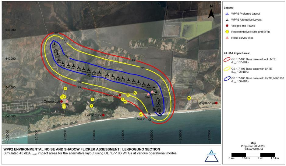
Figure 7-11: Simulated 45 dBA L<sub>A90</sub> impact areas for the WPP2 alternative layout, Lekpoguno Section | GE 1.7-103 WTGs
