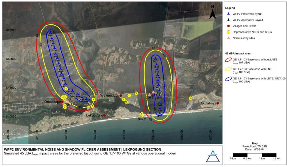
Figure 7-9: Simulated 45 dBA L<sub>A90</sub> impact areas for the WPP2 preferred layout, Lekpoguno Section | GE 1.7-103 WTGs
