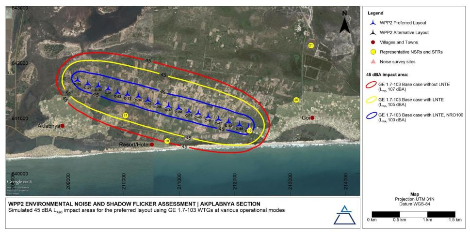
Figure 7-10: Simulated 45 dBA L<sub>A90</sub> impact areas for the WPP2 preferred layout, Akplabnya Section | GE 1.7-103 WTGs
