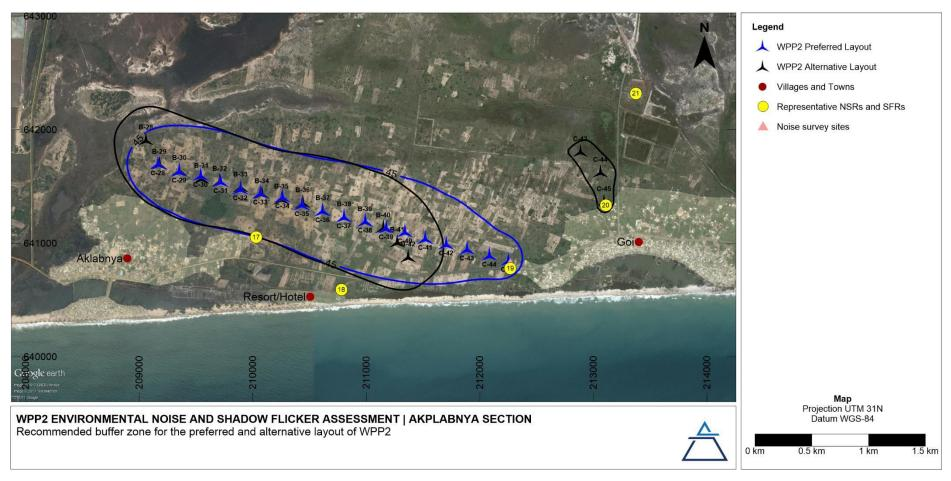
Figure 7-14: Recommended buffer zone for the Akplabnya section of WPP2, for noise impact mitigation and management.
