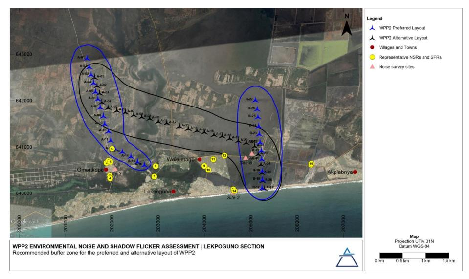
Figure 1: Recommended buffer zone for the Lekpoguno section of WPP2, for noise impact mitigation and management
