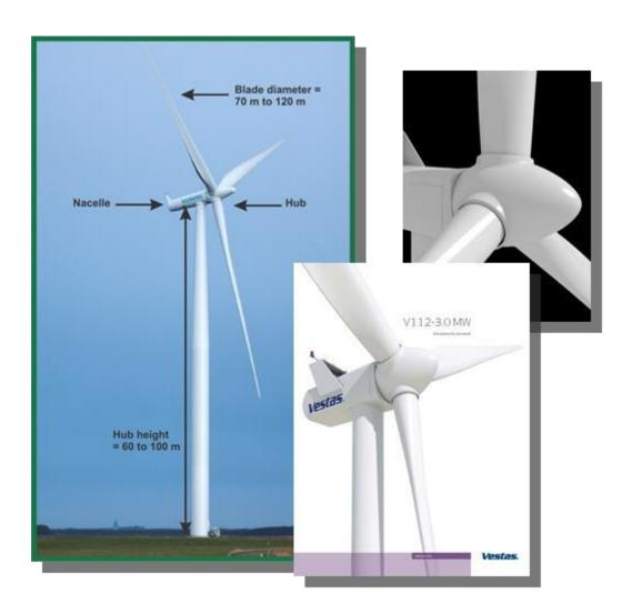
Figure 3-3: Illustration of typical wind turbines
