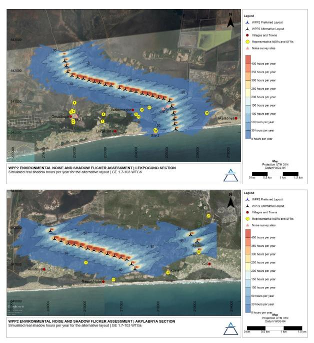
Figure 7-16: Simulated real shadow hours per year for the WPP2 alternative layout
