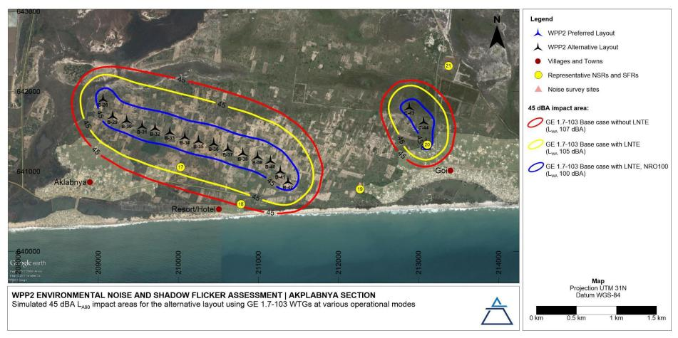
Figure 7-12: Simulated 45 dBA L<sub>A90</sub> impact areas for the WPP2 alternative layout, Akplabnya Section | GE 1.7-103 WTGs
