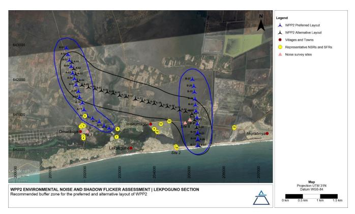
Figure 9-1: Recommended buffer zone for the Lekpoguno section of WPP2, for noise impact mitigation and management
