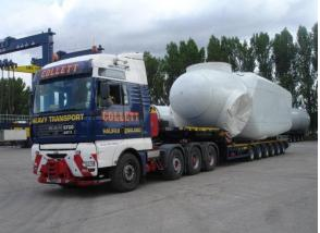
Figure 3-4: Transportation of a Nacelle
