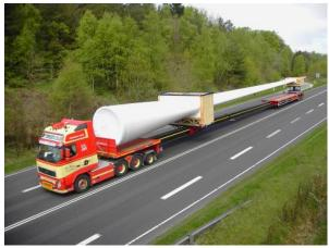
Figure 3-3: Transportation of a Rotor blade.
