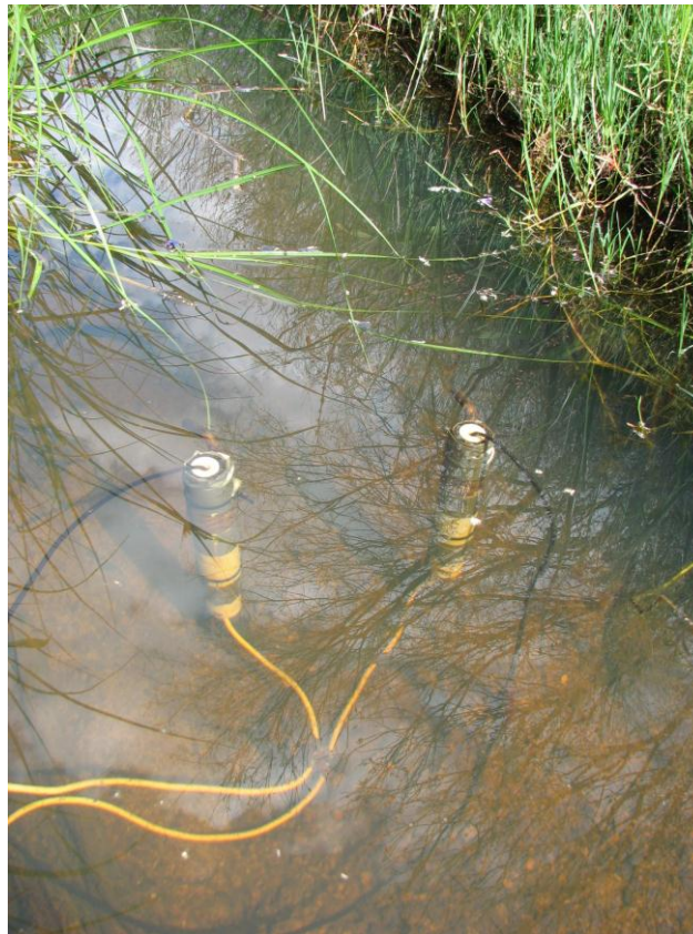
Figure 22 Oxygen and temperature loggers installed in a waterway
