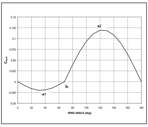
Figure 4-7. Sample Yaw Normalized Moment Coefficient
