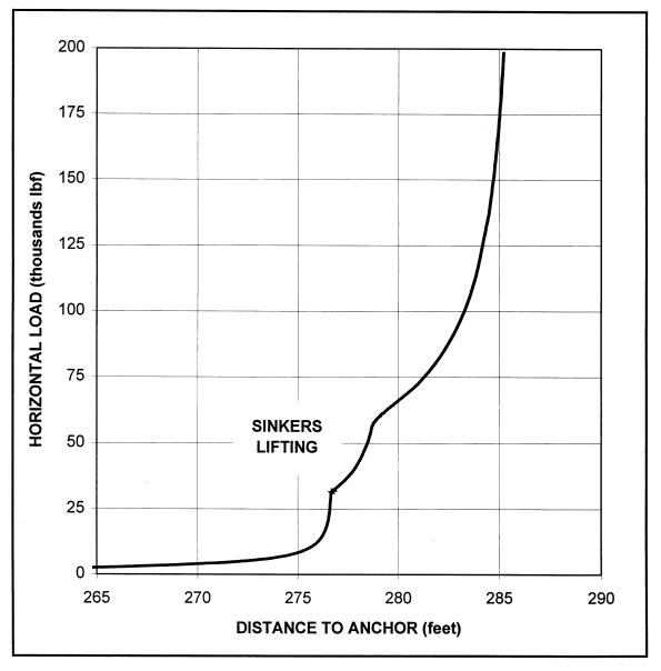
Figure 6-7. Load/Deflection Curve for the Example Mooring Leg
