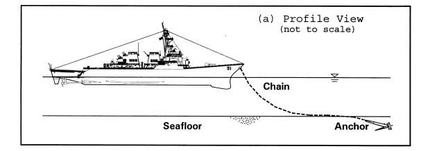
Figure 2-6. Ship at Anchor
