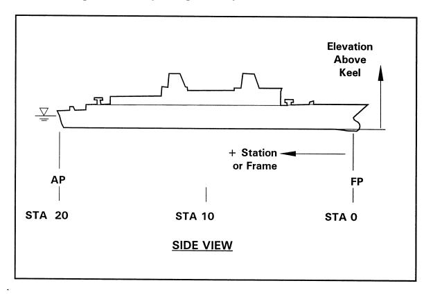
Figure 3-2. Ship Design and Hydrostatic Coordinates
