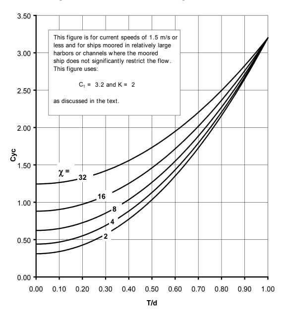
Figure 4-9. Broadside Current Drag Coefficient
