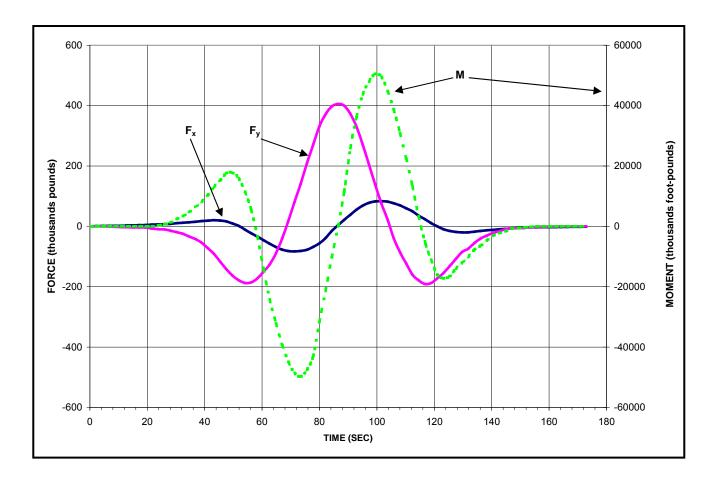
Figure 9-2. Example of Passing Ship Predictions
