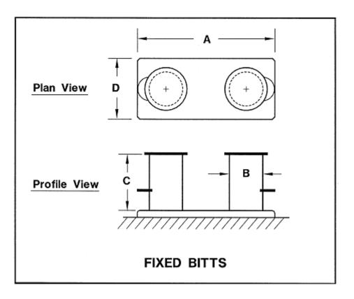
Figure 7-1. Ship's Fixed Double Bitts
