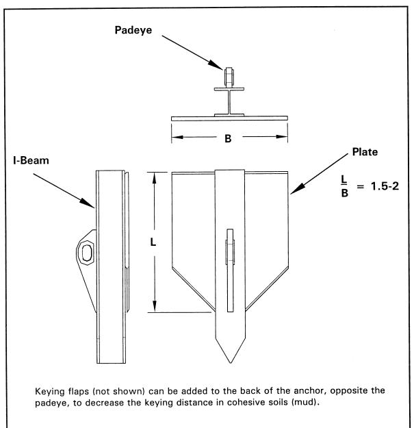
Figure 5-3. Driven-Plate Anchor
