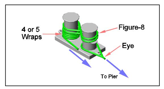
Figure 11-2. Securing Two Parts of Heavy Weather Mooring Line
