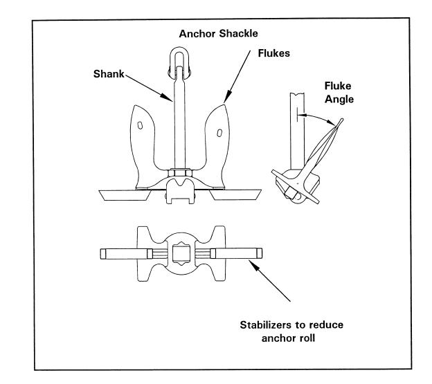
Figure 5-1. Example of a Drag-Embedment Anchor (Stabilized Stockless Anchor)
