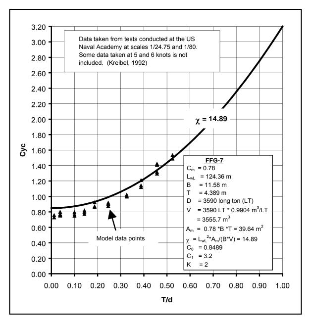
Figure 4-10. Example of Transverse Current Drag Coefficients
