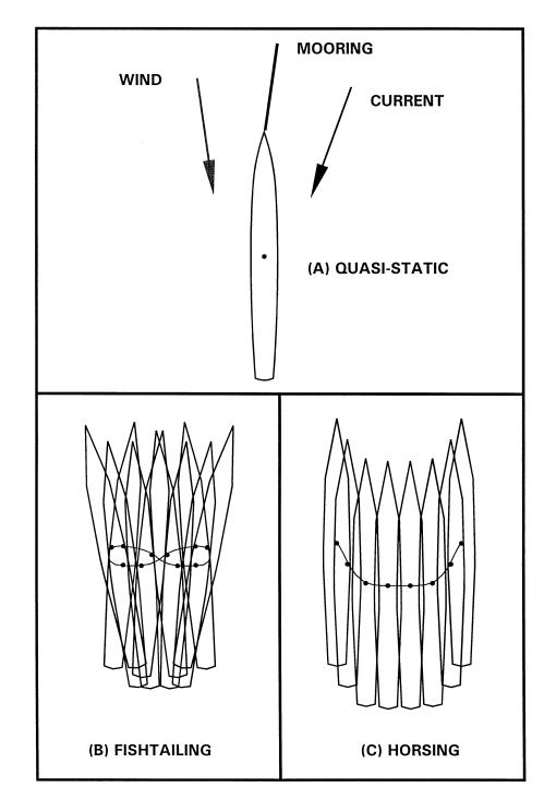
Figure 8-1. Some Types of Behavior of Ships at Single Point Moorings
