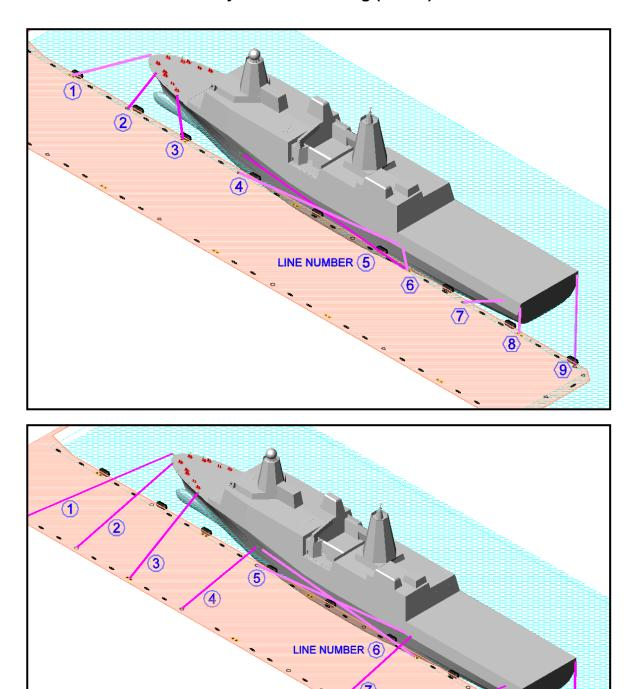
Figure 11-1. Example of a Standard LPD 17 Mooring (Upper) and Heavy Weather Mooring (Lower)
