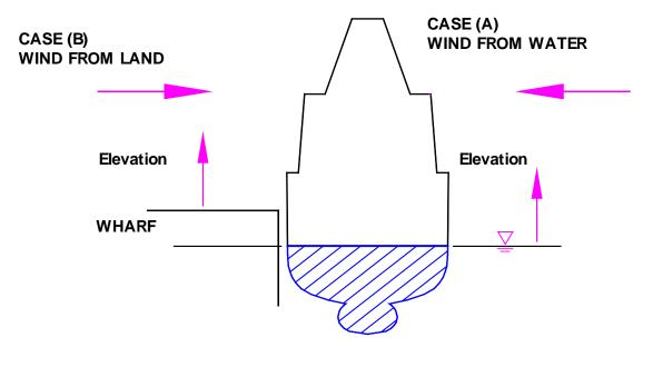
Figure 4-6. Blockage Effect for an Impermeable Structure Next to a Moored Ship
