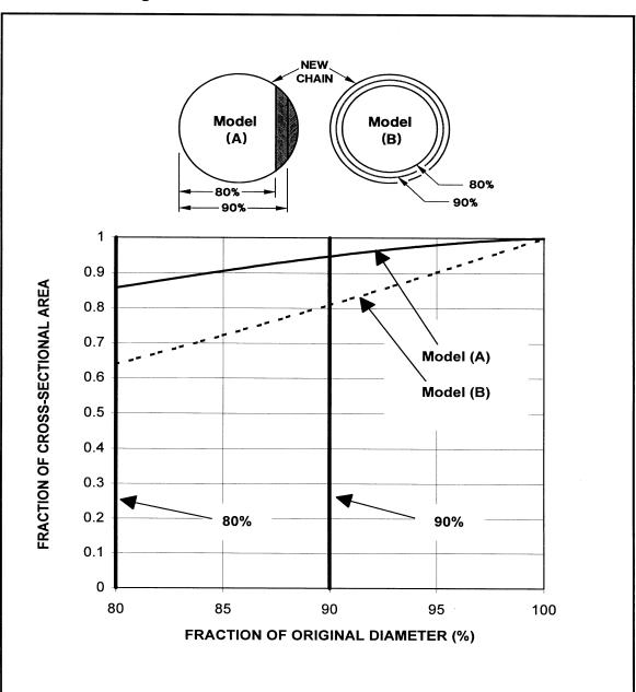
Figure 3-11. Idealized Models of Chain Wear
