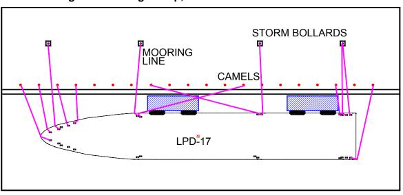
Figure 2-1. Single Ship, Offset From a Pier With Camels
