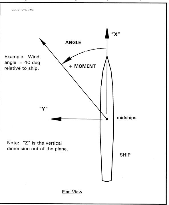
UFC 4-159-03 3 October 2005 Change 1, 1 September 2012 Figure 3-3. Local Mooring Coordinate System for a Ship
