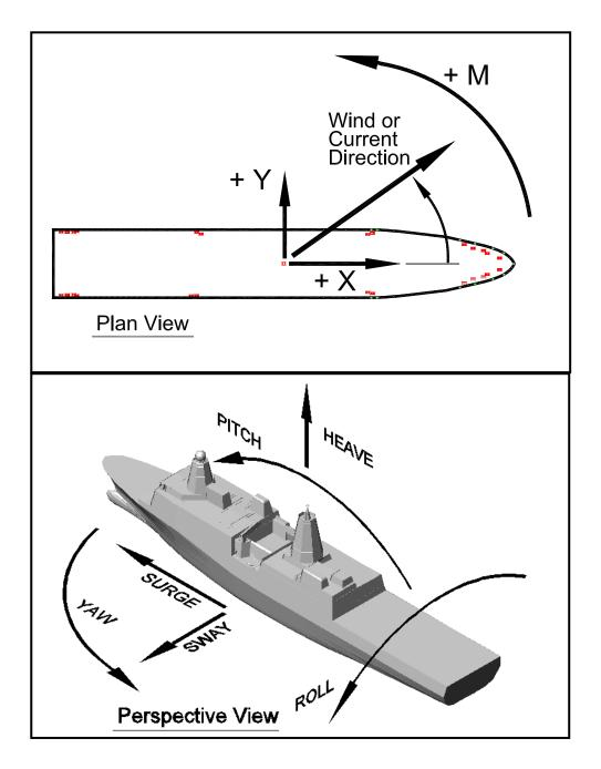
Figure 4-2. Local Coordinate System for a Ship
