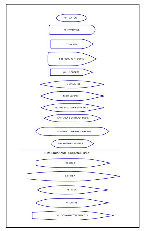
Figure 10-2. Ship Hull-Forms Tested (after Sorenson, 1997)
