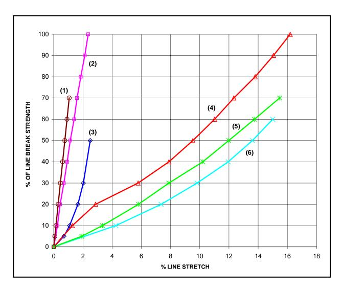
Figure 6-2. Synthetic Line Stretch
