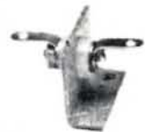
Fig. 3—Feedthrough insulator made from the nylon wheels of a curtain runner.
