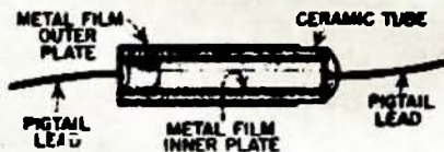
CERAMIC CAPACITOR CONSTRUCTION FIG. 4 A
