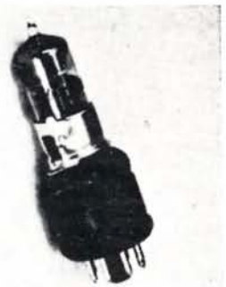
Fig. 1—A miniature-tube adapter for an octal socket.
