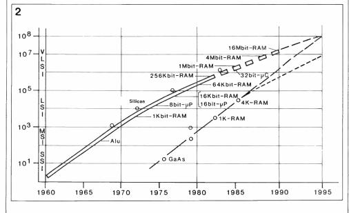
Fig. 2. The evolution and complexity of integrated circuits.
