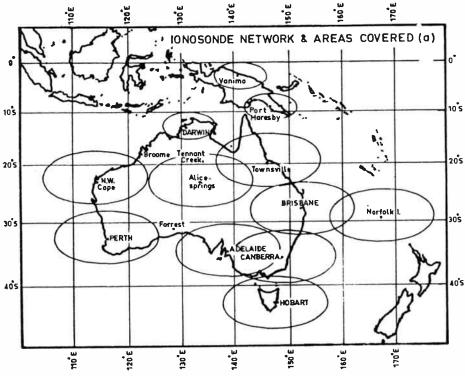
Figure 5. IPS Radio and Space Service plans to establish a network of ionsondes (IPS 5A) that will be remotely interrogated from Sydney to provide real-time ionospheric data to customers. The proposed distribution of ionosonde sites is shown here together with the geographical coverage achieved (G. K. Webster).
