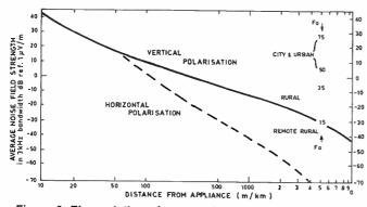
Figure 6. The variation of man-made noise with distance and antenna polarisation. Measurements were made at 5.5 MHz. Note the significant advantage offered by horizontal polarisatin with increasing distance from the interfering source. (R. T. Rye).
