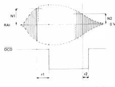
In DPSK mode 105 ms < t1 < 205 ms In FSK mode 215 ms < t1 < 315 ms
