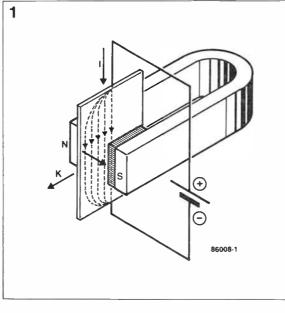
Fig. 1 The magnet pushes the electric current out of the area with maximum magnetic field strength.
