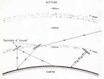
Figure 10. Effects of Es-layer tilts on HF-propagation depending on orientation and position of the layer relative to the transmitter. (A. K. Paul).
