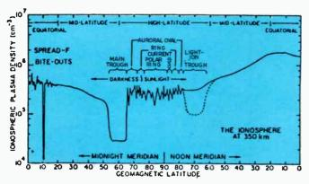
Figure 3. A perspective of phenomena in the ionospheric F-layer. The diagram is an idealised representation of ionospheric behaviour along a great circle path starting at the midnight equator, travelling north or south through the pole and returning to the noon equator. It represents the typical disturbances found along this path. The midlatitude region is fairly well behaved, but both the equatorial and polar ionospheres suffer considerable fluctuations. (E. Szuszczewicz et al).
