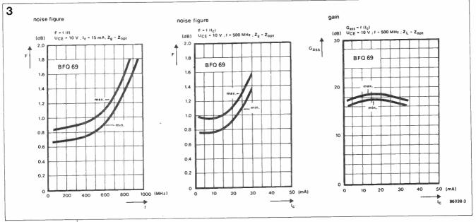
Fig. 3. Curves showing the characteristics of the new BFQ69 transistor. Note that the curves in Figures 3b and 3c refer to a test frequency of 500 MHz and not to the design frequency of the present preamplifier. (Siemens)
