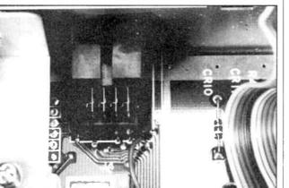
Fig. 9. Where to tap the +5 V supply for the interface. (Atari 1040-ST only).
