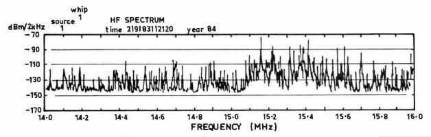
Figures 8. Signal levels in a 2 MHz segment of the HF band. This frequency range from 14 to 16 MHz covers both the 20m amateur band (14.00 to 14.35) where the average signal is low, and the 19m shortwave broadcasting band (15.10 to 15.45) where signals levels are as high as for any other single allocation class. (B. D. Ward).
