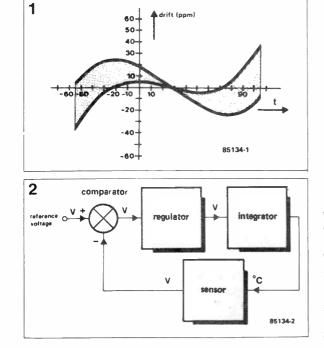
Of all the factors affecting the stability of crystal oscillators, temperature variation is the most detrimental. Therefore, where very good stability is required, the crystal is invariably fitted in a temperature-controlled oven.
