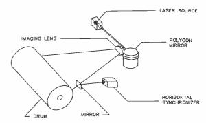
Figure 1. How the laser beam is scanned across the 'xerographic' surface of the drum. (Courtesy Impact Systems).
