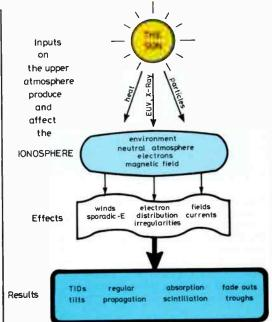
Figure 1. The ionospheric system (D. G. Cole).
