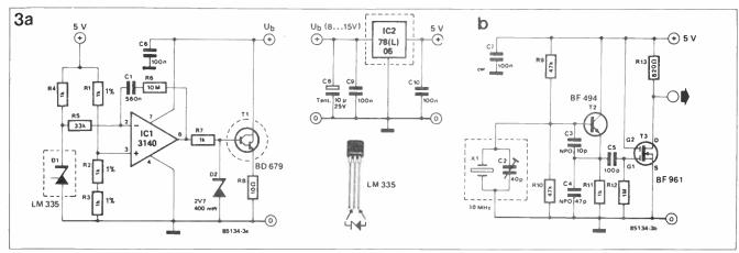
The 3140 will toggle when the output of the LM335 equals or exceeds the reference voltage of 3.330 V. For the sensor to provide this potential, the ambient temperature must be 60 °C (0 K + 333 K). When the opamp toggles, it switches off transistor  $T_{1}$ , a variable current source functioning as the heating element.
