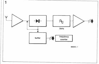
with a cut-off frequency of 5 kHz and then applied to an AF amplifier. The audio output is sufficient to drive a pair of headphones, but may also be used to drive a more powerful AF amplifier.
