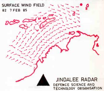
Figure 13. Surface wind direction map for North Western Australia computed from the Jindalee OTH radar backscattered signals. This was the first such map transmitted from the Jindalee project to the Bureau of Meteorology and represents a world first in providing a national weather service with access to HF radar synoptic remote sensing data. (S. J. Anderson).
