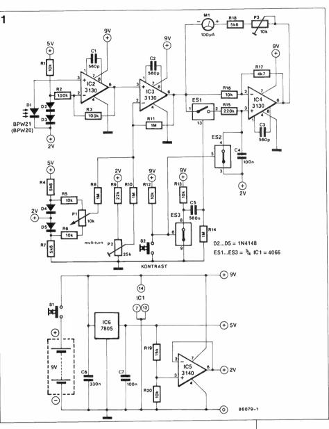
mounted in a manner which ensures that the light from the enlarger reaches it freely. Diodes  $D_2$  and  $D_3$ should be placed as close as possible to the photodiode, so as to keep temperature differences between the three as small as possible.
