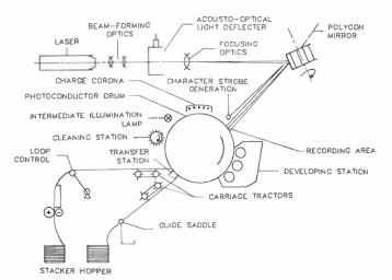
Figure 2. Schematic diagram of the laser electrophotograph process. (Courtesy Impact Systems).
