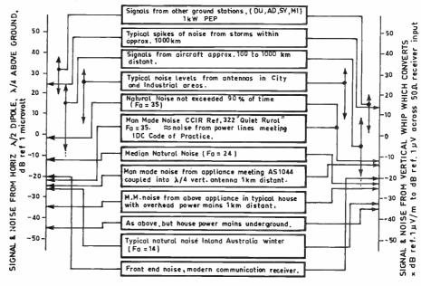
Figure 7. Comparative noise and signal levels measured at Melbourne airport on 5.5 MHz at midday. Note that signals from distant aircraft are below the noise levels experienced from antennas located in city and industrial areas. (R. T. Rye).
