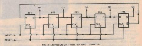
Q output, but from its Q-bar output. This introduces a logical inversion or "twist" into the ring, because the first FF must always adopt the opposite state from that of the last.
