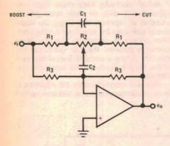
Fig. 1: typical octave equaliser section.
