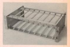
A new type of rack-mounting frame for plug-in PCB assemblies is available from Celotek Industries. Designed to mount in a standard 483mm (19-inch) rack, the frame is capable of mounting up to 16 PCB modules on 25mm centres.
