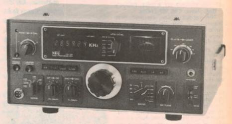
The digital frequency meter readout is to the left of the upper panel, with the VFO/XTAL switch and monitor meter to the right. The lower controls are, L to R, Mode, Rx Gain, Tx Gain, Band, RF Tune, and PTT/VOX, etc.
