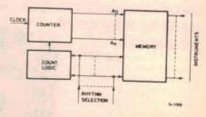
The block diagram of a basic rhythm generator is shown above. All this is contained in the M252.
