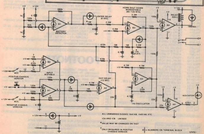
Circuit diagram of the complete alarm system. The four operational amplifiers in each LM3900 are shown as separate devices, identified as A1, A2, etc; B1, B2, etc. Note that most
