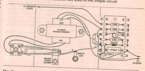
This diagram and the photo below show how to assemble the unit.
