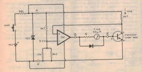
The op-amp provides base current for the transistor under test, whose action causes equal voltages to occur at the op-amp-input terminals. If Vref is 5.3V, sufficient base current will flow to provide 1mA collector current. Gain of the transistor is then 1mA/base current, and the meter scale is calibrated. Thus, the 50uA point is marked 1000/50 = 20, and so on. A gain value of 400 is marked
