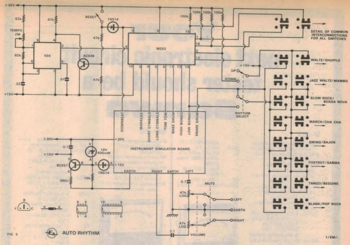
This circuit diagram shows how the M252 is interfaced to the player and to the instrument board.
