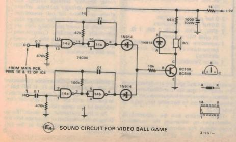
frequency of 1kHz, and the resulting sound can be described as a "ping". In a similar fashion, the second oscillator is gated on when the ball strikes the left bat, but this time, since the oscillator frequency is lower, a "pong" is produced.
