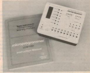
module is designed to demonstrate, using the SBP 0400 device as an example. Each of the control inputs, data inputs and data outputs of the device are brought out the LED indicators, and all inputs are provided with miniature toggle switches so that the device may be manually programmed. A pushbutton provides the clock signal input.
