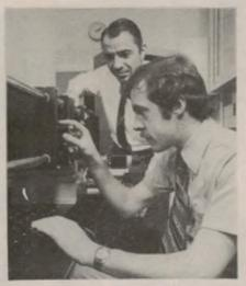
it optimizes detection of the very weak Raman signal from the particle of interest in a sample and minimizes all other sources of interference. The entire instrument is connected to a minicomputer which allows automatic data acquisition over a long period of time.
