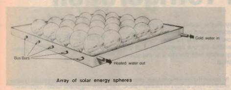
A major challenge facing solar cell manufacturers is to reduce the cost of their cells relative to the electrical output, both by increasing cell efficiency and by reducing manufacturing costs. One interesting new development, aimed at improving efficiency, is a revolutionary solar panel that automatically tracks the Sun, and yet has no moving mechanical parts.
