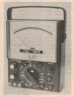
where it was within 2%. Similarly, on the AC voltage scales, accuracy was within 2% of full scale. Resistance measurements were also within 2% using 500 as FSD. Midscale reading on the ohms scale is 20 so the meter is useful for resistance measurements down to a fraction of an ohm.
