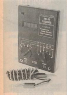
University Graham Instruments Pty Ltd, 106 Belmore Road, Riverwood, NSW have released the Kamoden HM-35 digital multimeter which had 3½ digit readout and 10M input impedance on all ranges. Range switches are similar to those on a conventional meter.
