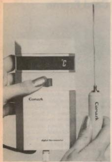
The Comark 3001 is a small hand-held digital thermometer which enables fast, accurate temperature measurements from -50°C to +800°C. It is battery powered and weighs 300 grams.
