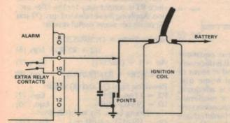
FIG. 3 DISABLE IGNITION CIRCUIT
