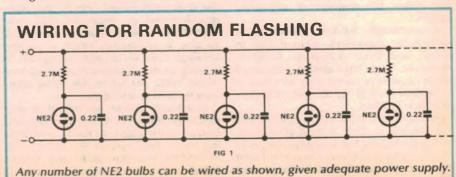
capacitor faster than it can be charged through the 2.7M resistor. When the voltage falls to about 55, it can no longer maintain ionisation; the bulb ceases to glow and to draw current, and the charging cycle begins all over again.
