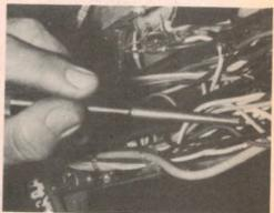
**4.18pm** "This wiring's a real birds nest. Passed through the wires with the Minispeed stone cold, desoldered the three joints, let the iron cool down, then withdrew through the PVC insulation. The 5 second heat up and low tip mass let's me do this".
