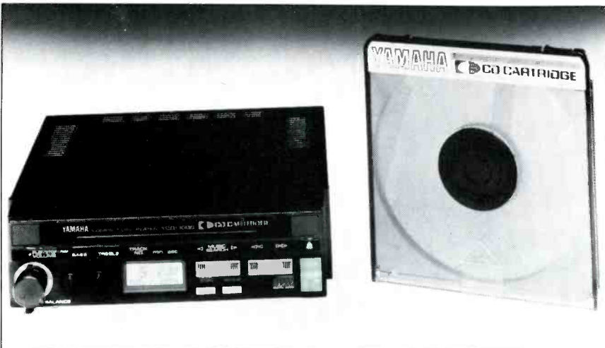
Yamaha's YCD-1000 loads CDs in cartridges.
