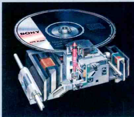
Sony Linear Motor Tracking System
