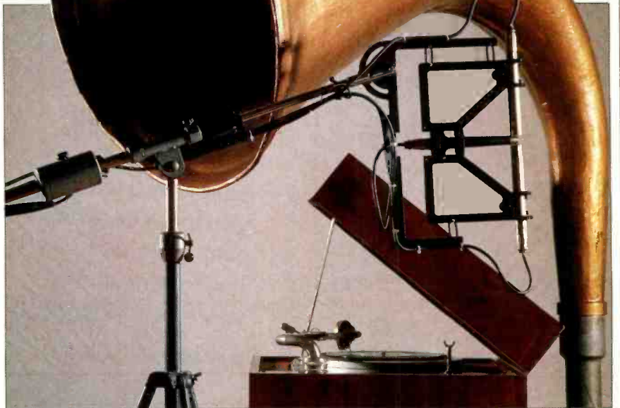
The microphone system and player used in Nimbus' Natural Ambisonic Transfer system.
