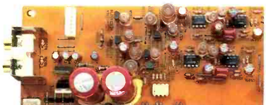
3rd-order analog filters cause less phase shift than the 7th- and 9th-order designs that others use.
