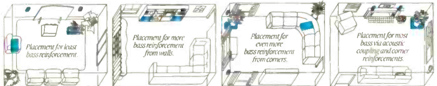
You can put Ensemble's low-frequency units exactly where they should go for superb bass. You can't do this with conventional speakers because you have to be concerned about the upper frequencies coming from the same enclosures as the low ones.
