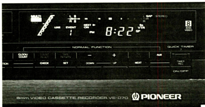
MOST OF THE SECONDARY CONTROLS ARE GROUPED TO THE RIGHT SIDE OF THE VCR. BELOW THE STATUS DISPLAY, WHICH, AMONG OTHER THINGS, INDICATES WHICH TRACK IS BEING PLAYED OR RECORDED IN THE PCM-MULTI MODE.
