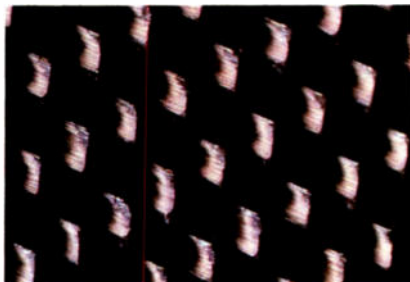
Lightweight, yet rigid, carbon fiber eliminates breakup, flexing and distortion in woofer cones.
