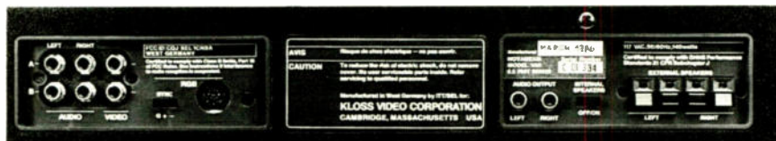
BACK PANEL OF THE NOVABEAM 100 PROJECTOR, WITH STEREO AUDIO AND VIDEO (COMPOSITE AND RGB) INPUTS AT LEFT AND LINE- AND SPEAKER-LEVEL AUDIO OUTPUTS AT RIGHT
