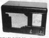
SHELLEY RADIO CO. - This "Commuter" radio, manufactured in Los Angeles, Ca., around 1937, features an Art Deco Bakelite front, but the rest of the cabinet is wood. The Golden Gate bridge and San Francisco Bay are drawn on the translucent celluloid dial. The grille cloth is not original. (Adam Schoolsky - Fremont, CA)
