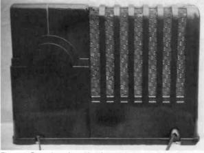
Figure 2. Rear view of the Model 4500. Note that the speaker grille wraps from the front of the radio across the top and down the back.
