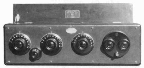
Figure 1. The Atwater Kent Model 21 dry cell set with the cover lid open to show the unique metal tag.
