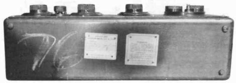
Figure 3. Bottom view of the Atwater Kent Model 21 showing the two manufacturer's labels. To the left is the model number label, and to the right is the warranty tag.
