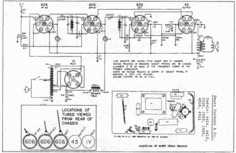
Figure 3. Schematic and parts layout from M.N. Beitman, "Most Often Needed Radio Diagrams, 1926–1938."
