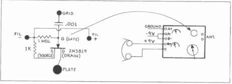
Figure 2. Schematic of the wooden WD-11, detail on the FET and battery connections for the Radiola Senior, a later version of the Aeriola Senior.
