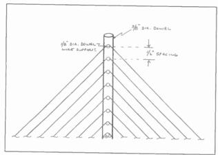
Figure 2. Partial view of a diamond loop showing construction detail.
