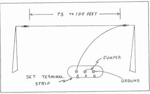
Figure 5. Diagram for a single wire antenna system.
