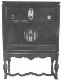
RCA RADIOLA MODEL 18 - This is a 1927 seven-tube TRF set in a custom hardwood cabinet with folding doors. The lid of the cabinet opens up for easy access to the chassis. (Bill & Barb Graham - Aurora, NE)
