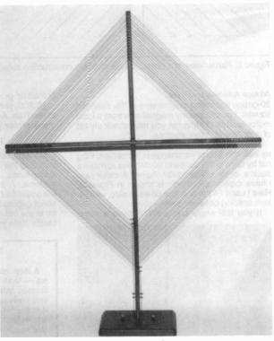
Figure 1. A typical diamond loop antenna.
