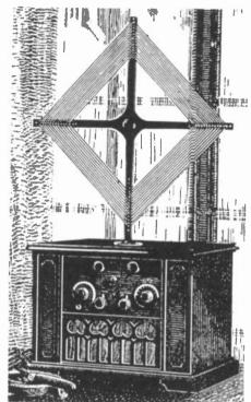
Figure 3. This DeForest D-12 Radiophone Special, a 5-tube set, 1925, "with a DeForest loud-speaker of exceptional tone quality built into the cabinet, ...can be readily picked up and moved."
