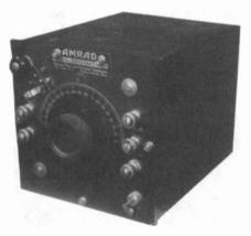
AMRAD TYPE E CRYSTAL SET - This set does not have the magnetic type detector, which may mean it is an older model. Note the detector in the lower right-hand corner. I also have the matching amplifier. (Paul Giganti - San Carlos. CA)
