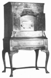
GENERAL MOTORS MODEL 150 - The woods used in this floor model are exceptional! This 1930 TRF set has eight tubes. The speaker faces the floor and a phonograph is revealed when the top is lifted. (Kurt Thompson - Jacksonville, FL)
