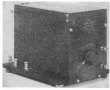
Figure 2. 1-tube detector set with a "telephone receiving radius of approximately 75 miles."
