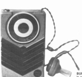
AIWA AR-150 - This Germanium radio is typical of the plastic-style, Japanese sets of the early 1960s. It is equipped with a small earphone. (Erwin Macho - Vienna, Austria)
