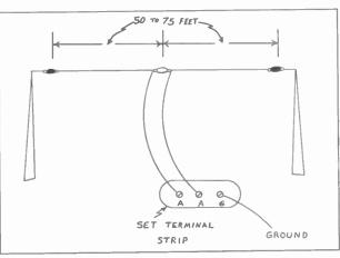
Figure 4. Diagram for a doublet antenna system.
