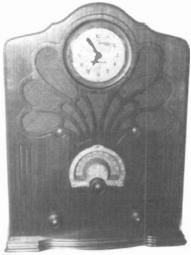
BULOVA MODEL M-701 - A feature of this set is an adjustable timer to turn the radio on and off. This 1932, 7-tube, 175 Kc, IF model was purchased in poor condition at a farm auction in South Dakota. It still needs a glass and bezel for the clock. (Scott H. Timperley - LeMars, IA)
