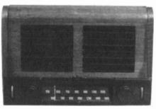
HOWARD MODEL 906 - The most noteworthy feature of this 1946 set is the use of a 6" x 9" oval speaker. The radio uses (2) 6SK7s, (1) 6SA7, (1) 6SQ7, (1) 6V6 and (1) 5Y3 type tubes. Although this AC set is AM only, it was made also with shortwave bands and vibrator battery power supply. (Doug Burskey - Mansfield, OH)
