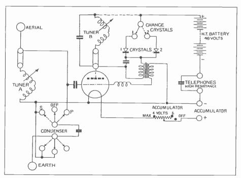
Figure 4. Circuit Diagram of the B.T.H. Valve-Crystal Receiver, Type VC. (Source: H.M. Dowsett, "Wireless Telephony and Broadcasting Volume II," copy courtesy of C.F. Crandell.)
