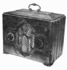
AIRLINE MODEL UNKNOWN – This 5-tube mantel radio appears to be circa 1933. Its tube complement is (1) 6C6, (2) 6D6, (1) 43, and (1) 25Z5. It has a heater strip resistor mounted to the back of the chassis instead of a line cord resistor. {Robert and Shirley Schafbuch – Carrollton, KY
