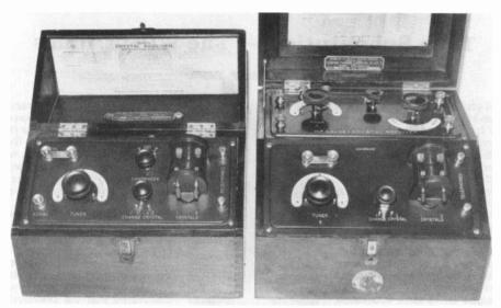
Figure 3. The Type VC, Form 'B' Receiver, right, and the earlier Radiola Type C Crystal Set, left. Note the similarity of the front panels.
