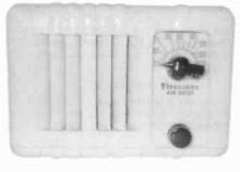
FIRESTONE AIR CHIEF MODEL S7425-4 — The dimensions of this tiny, white plastic set are 61/2" wide x 41/2" high x 41/2" deep. Manufactured ca. 1938, the set uses Types 6K7, 6J7, 25L6, and 25Z6 tubes, plus a resistance line cord. (Stanley Lopes — Concord, CA)
